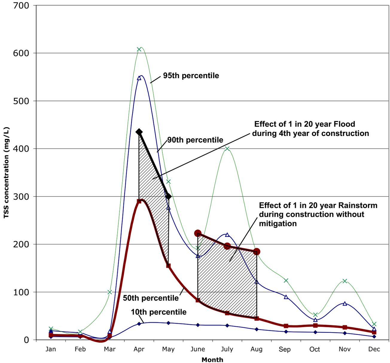
**Maximum Effects of Floods or Rainstorms During Construction on Sedimentation Concentration at Lockport**
