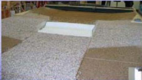
Hydraulic testing on the floodway outlet control structure model at the Hydraulics Research and Testing Facility at the University of Manitoba
