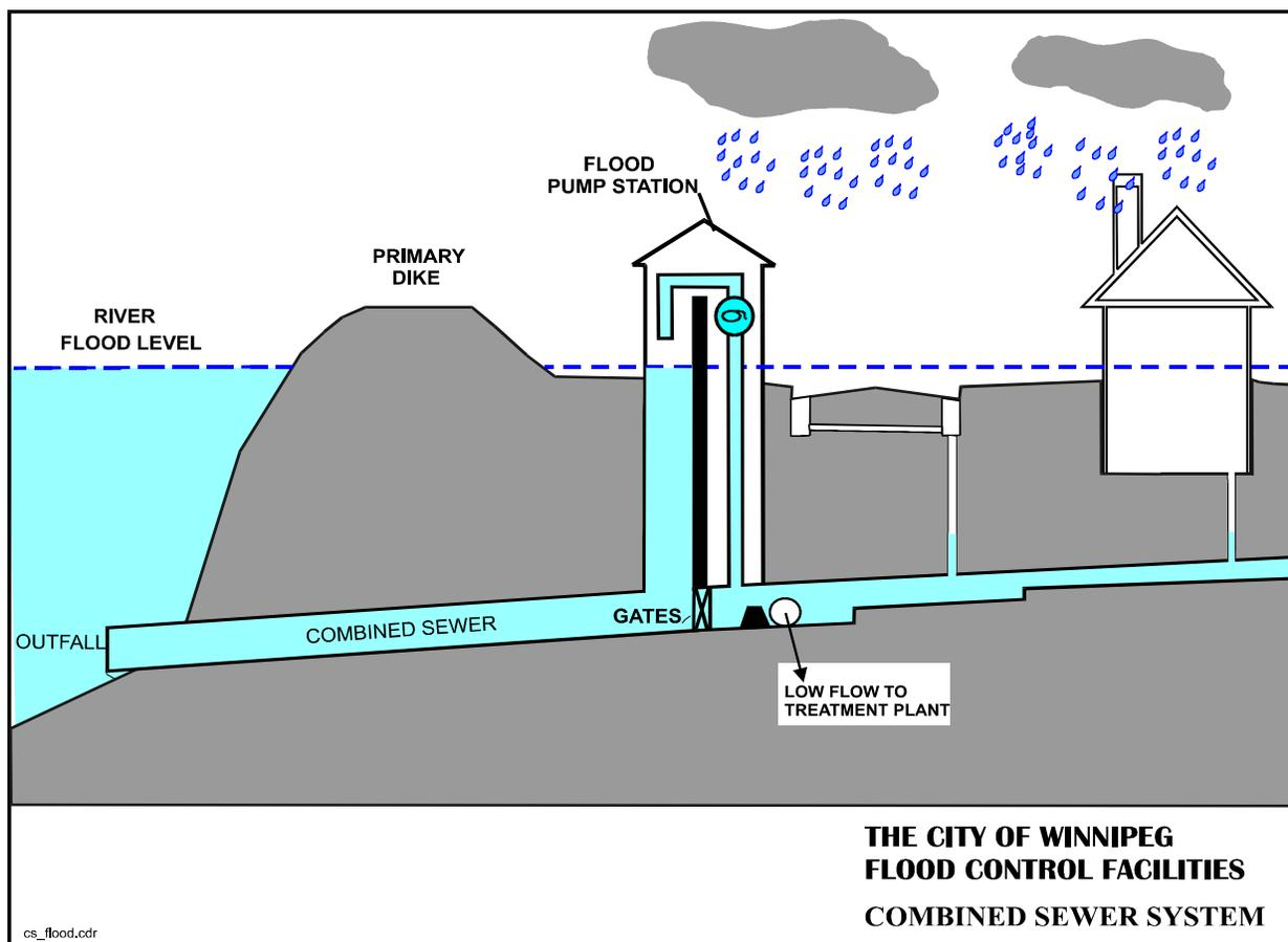
In the south end of the City where water levels exceeded 24.5 feet equivalent at James Avenue, the river water rose to a point that it backed up into the un-gated land drainage sewers, channels and creeks. The river water therefore surcharges to the point that it and land drainage flow (when raining) will pond
