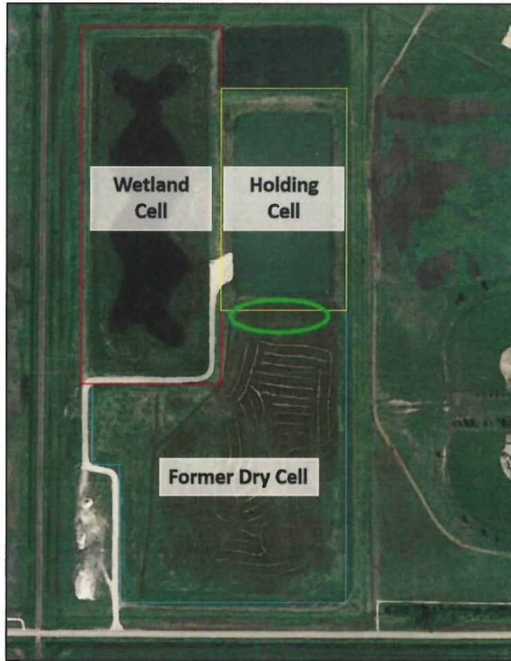
**Figure 1.** Aerial view of the Niverville Lagoon decommissioning project, including the former dry cell (licence removal December 2015), wetland cell (currently under licence) and holding cell. Green oval indicates approximate location of willow plantings in 2018. Image courtesy of Google Earth (Imagery date: 2015).
