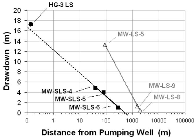
$$T_{LS} = \frac{2.3Q}{2\pi(\text{slope}_{LS})} = 8.7 \cdot 10^{-4} \text{ m}^2 / \text{s}$$
