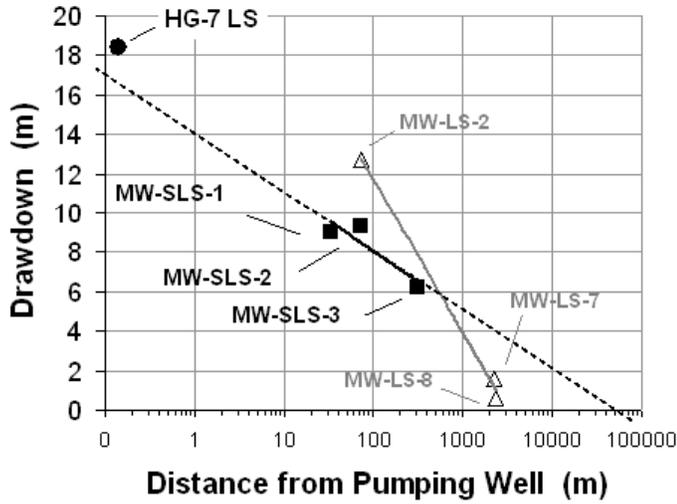
$$T_{LS} = \frac{2.3Q}{2\pi(\text{slope}_{LS})} = 2.7 \cdot 10^{-3} \text{ m}^2 / \text{s}$$
