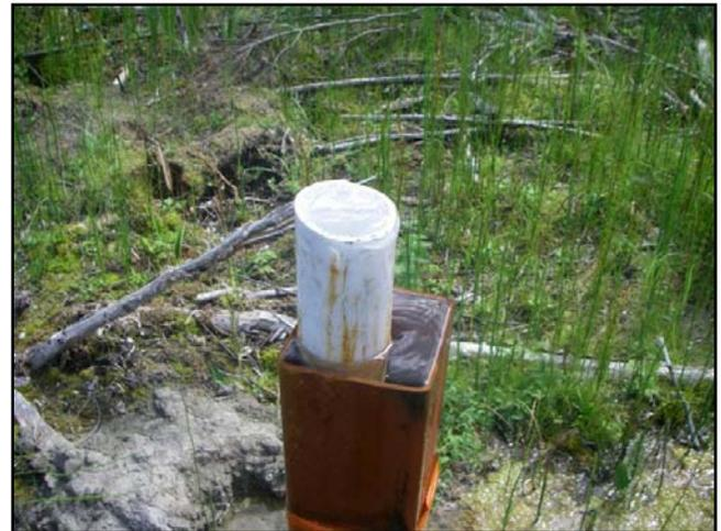
D. Flowing artesian conditions at MW-7-LS.
