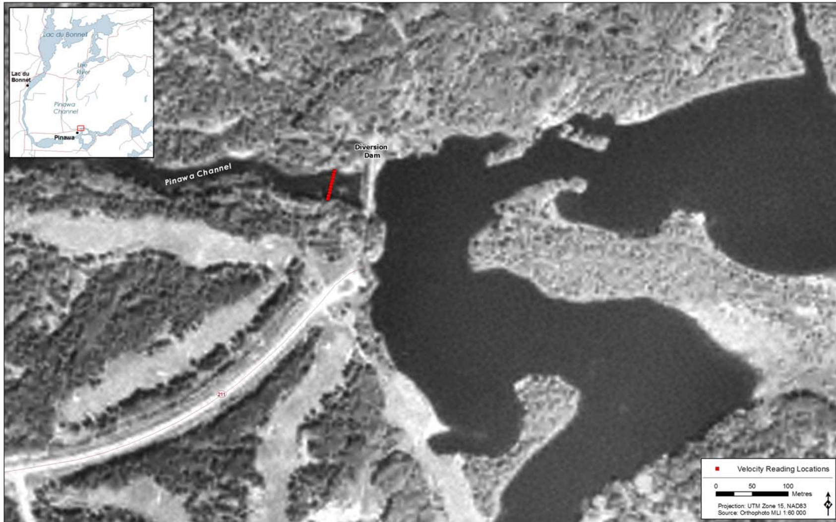
Figure A1. Cross section of the Pinawa Channel downstream of the Pinawa Diversion Dam where sectional discharges were measured in order to calculate total channel discharge.
