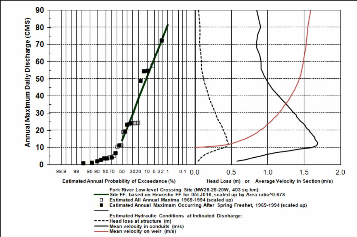
Figure 1. Estimated annual discharge exceedance frequency and estimated hydraulic conditions corresponding to the range of Fork River discharge conditions at RM of Mossey River low-level crossing replacement site, NW 27-29-20W.
