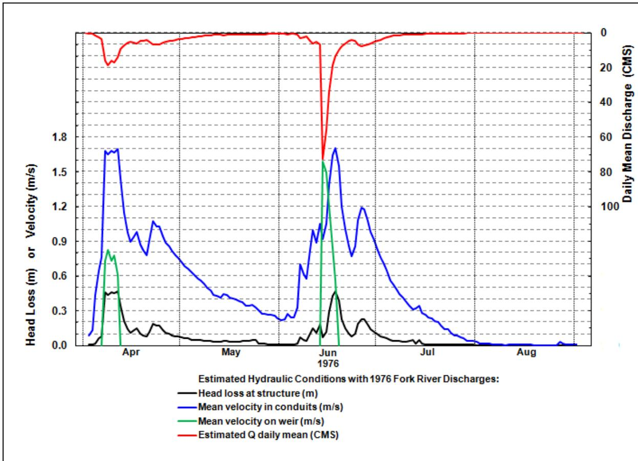
Figure 2. Simulated daily sequence of hydraulic variables at RM of Mossey River low-level crossing site, **NW 27-29-20W**, on basis of proposed crossing replacement geometry and estimated 1976 Fork River discharge hydrograph.
