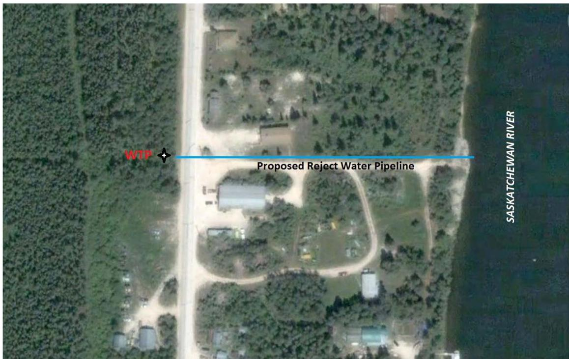
FIGURE 2.1 - PROPOSED MEMBRANE CONCENTRATE DISCHARGE ROUTE
