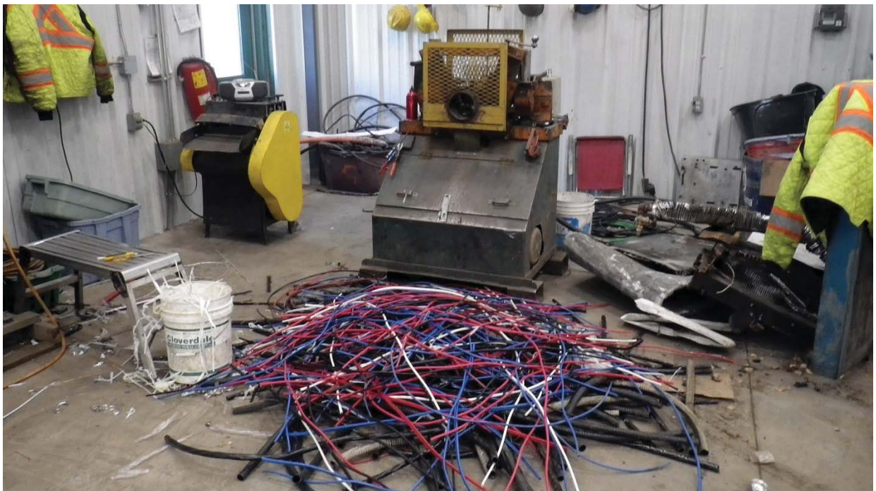
Photo 10 – Wire stripper and waste insulation from copper wire
