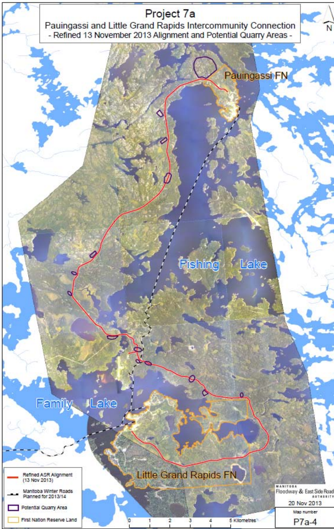
Figure 15. Locations of Rock Quarries and Borrow Areas Along the Road Right-of-Way Between Pauingassi and Little Grand Rapids First Nations
