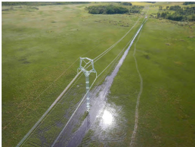
Photograph 4-1a. Rutting in wetland at site WET-197.
