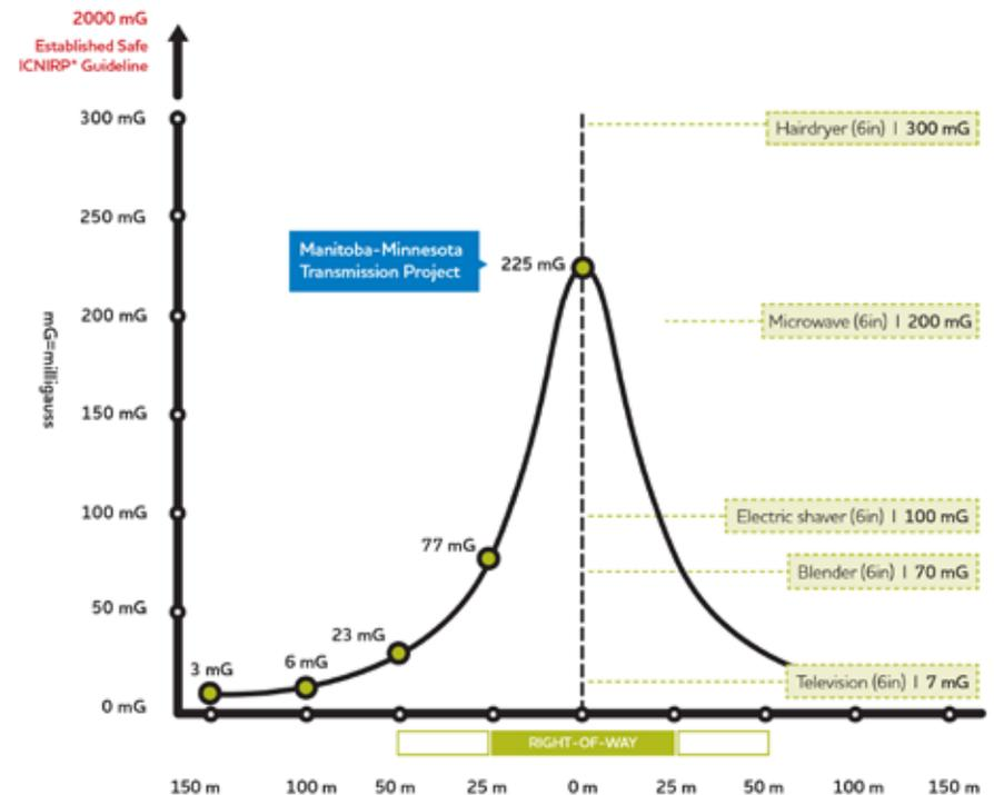
This figure represents magnetic fields 1.0 m above ground for a preliminary 500 kV line design.
