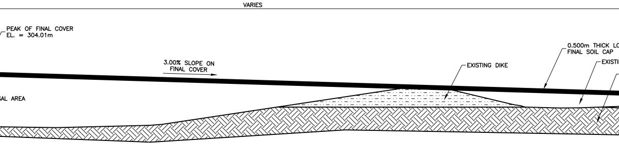
1 TYPICAL CROSS SECTION DETAIL 2 4 SCALE = 1:250
