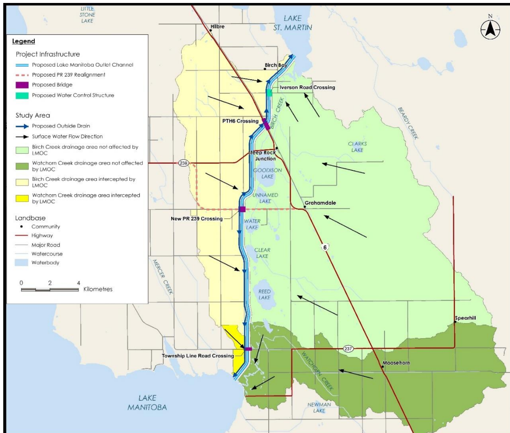
Figure 3C-14 LMOOC Permanent Drainage Plan
