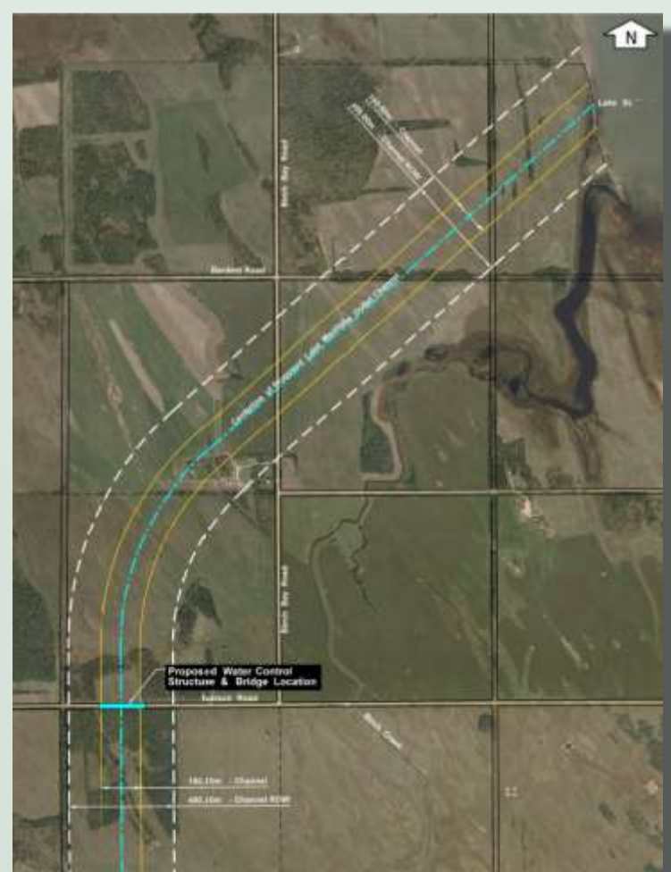
Iverson Road Water Control & Bridge Structure
