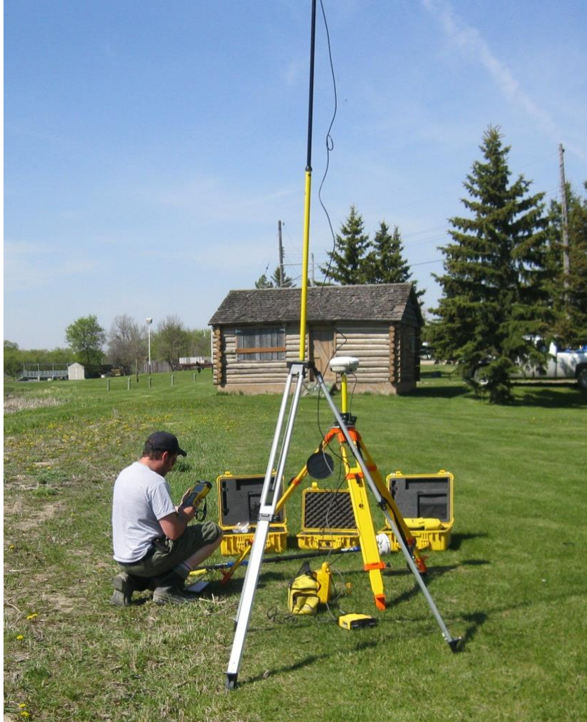
Figure A2-1. Photograph showing the setup of the real-time kinematic (RTK) GPS based acoustic habitat survey.
