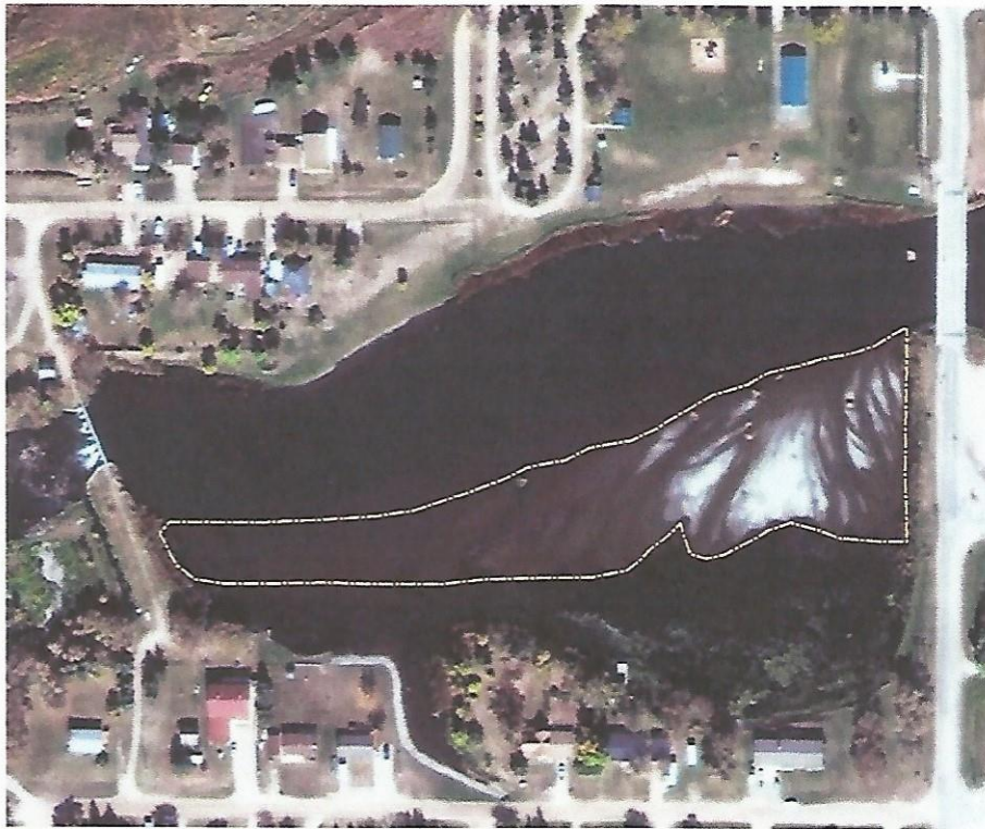
Figure 5-1. Large area of sedimentation outlined along the southern extent of the Little Saskatchewan River channel visible in a Quickbird high-resolution multispectral image from fall 2010 (O DigitalGlobe).
