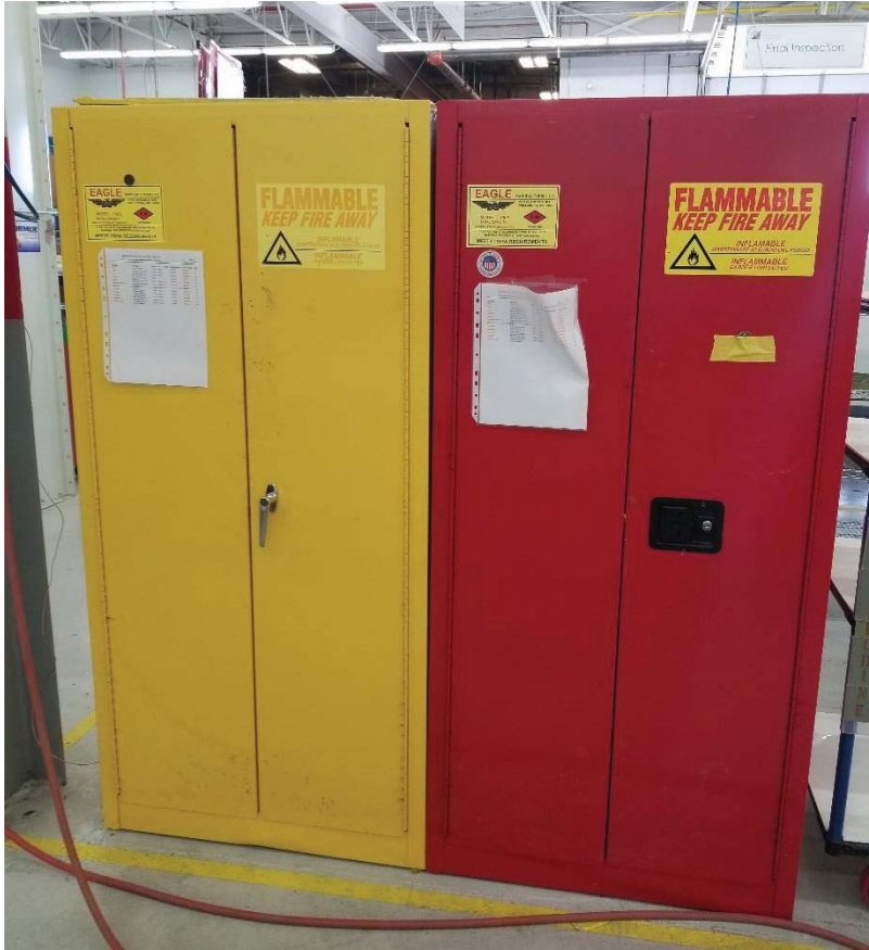
Photo B-11: Flammable materials storage cabinets
