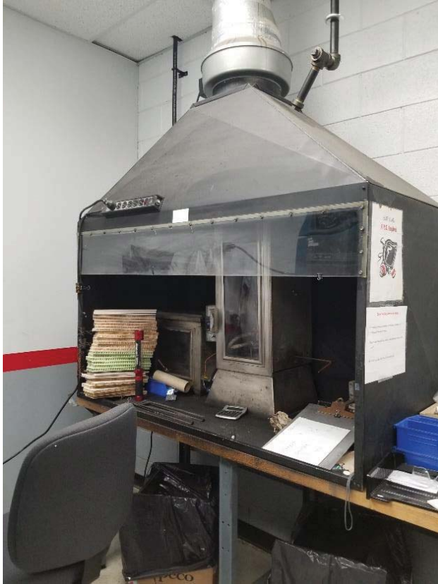
Photo B-7: Flammability lab fume hood, with samples stacked
