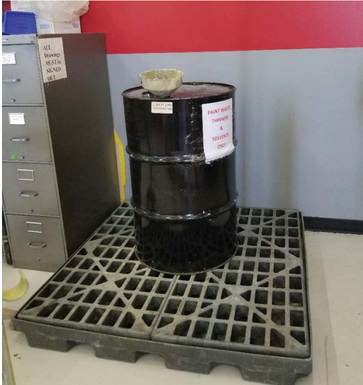
Photo B-23: Spill containment pallet for waste paint
