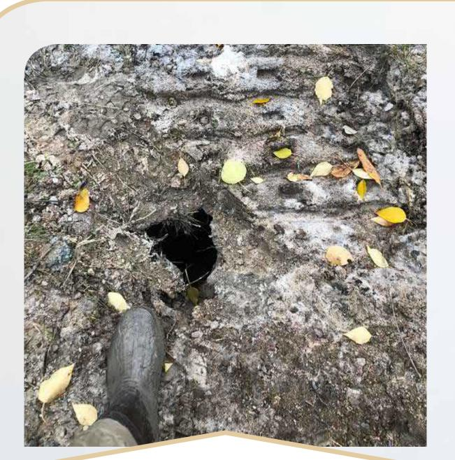
The holes (15-cm wide) collapse on themselves after drilling is complete and the core is extracted.
