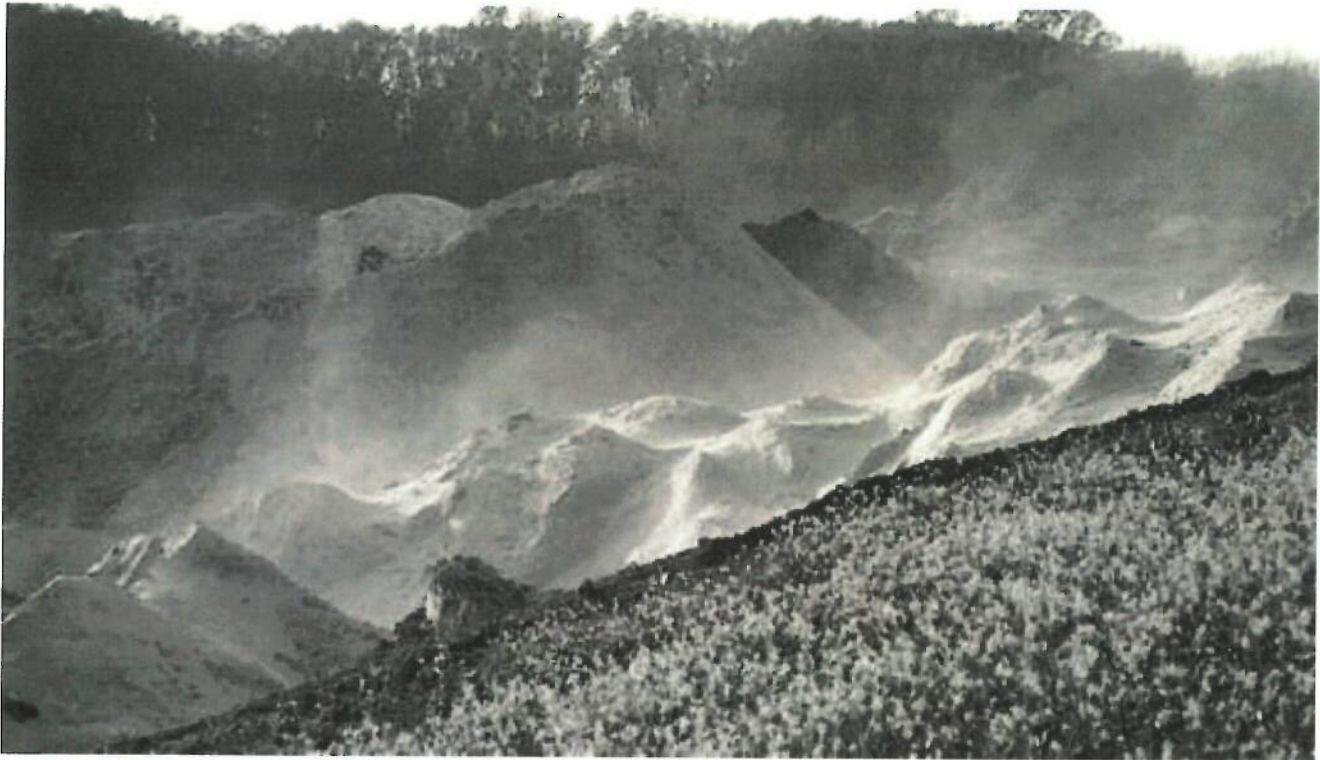
Figure 9 Silica dust blowing from stockpiled sand in Bloomer Wisconsin
