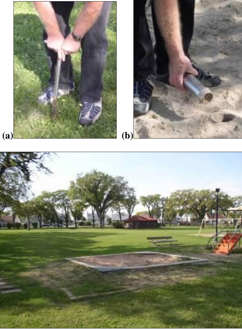
Figure 7. Collecting soil and sand samples. (a) sampling soil using a 2 cm diameter Oakfield soil sampler; (b) sampling sand from a sand box using a 5 cm diameter sampler; (c) a typical playground with grassed area, sand box, swings, and play structure.
