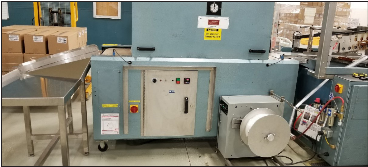
Photo B-31: Heat tunnel in a cartoning line used for shrink wrapping in the packaging area.
