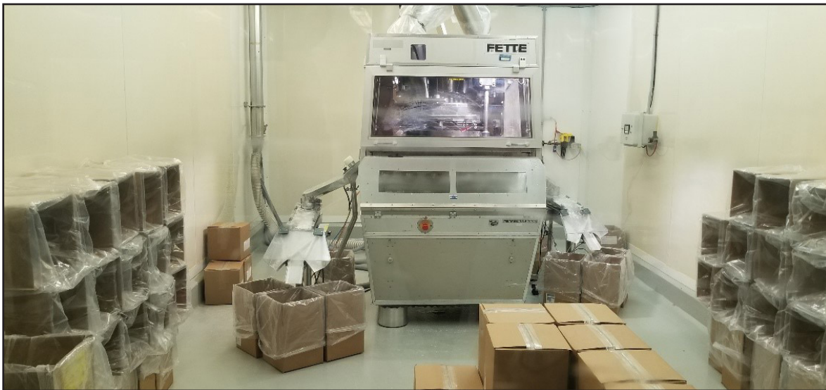
Photo B-26: Automated pressing machine in the compression section of the manufacturing area.
