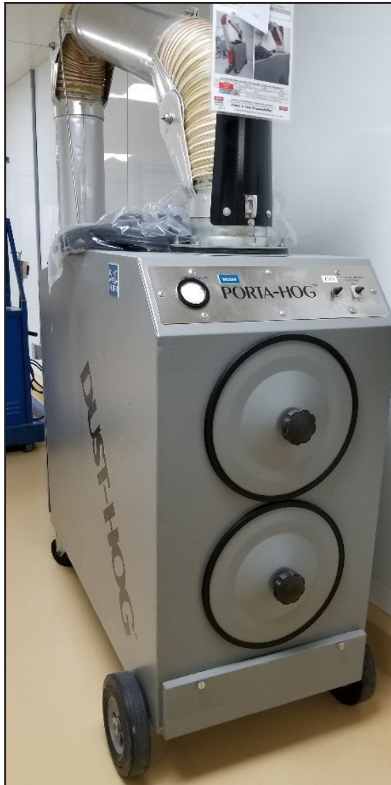
Photo B-35: Portable dust collector, located in the manufacturing area.
