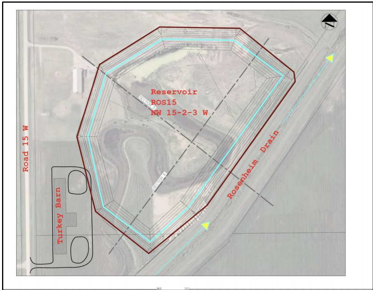
Figure 2 – Preliminary Layout Map for Preferred Location of Potential Water Storage Site ROS15 Adjacent to Rosenheim Drain in NW 15-2-3 W
