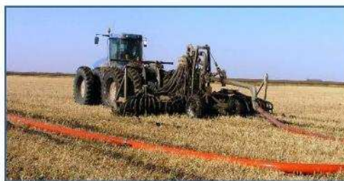
Figure 5. Example of manure injection technology.
