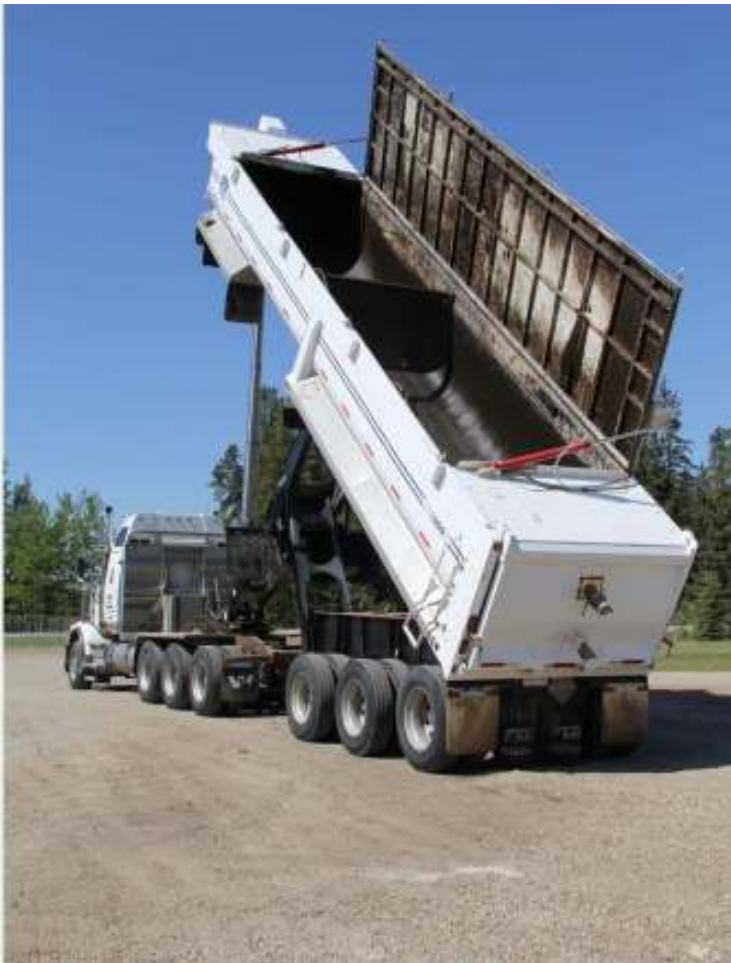
Figure 2. Sealed Lid End Dump truck for hauling peat http://cornerstonetransport.ca/services/#tab-f97f840907a6890d239
