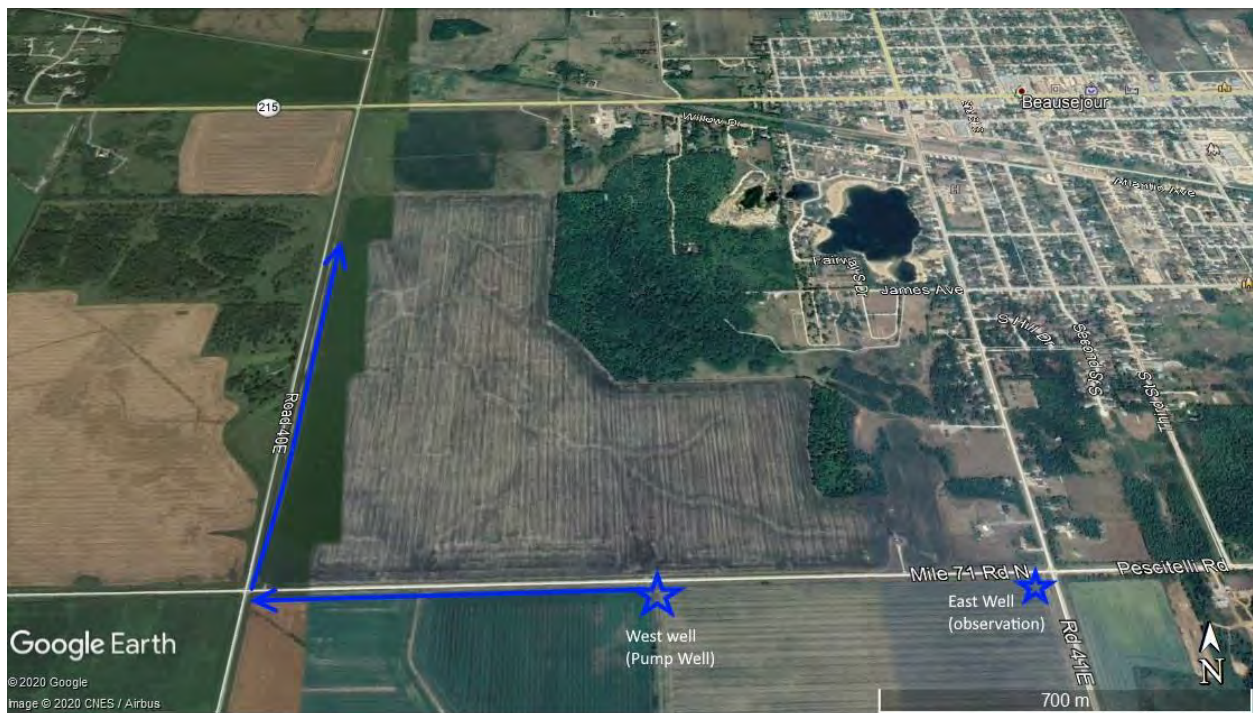
Figure 22 – Drainage Routing During 72-Hour Pump Test
