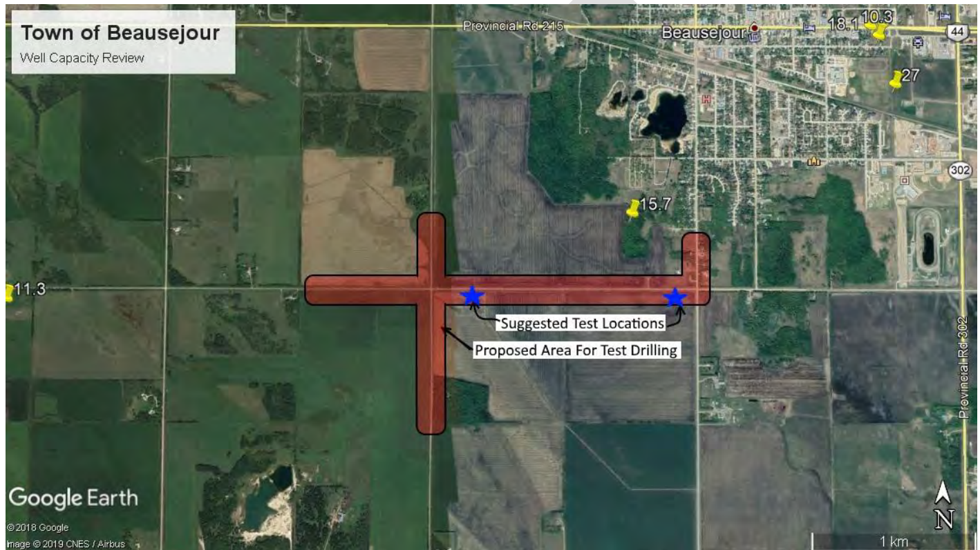
Figure 3 – Proposed area for test drilling within the road allowance; Yellow plotted points indicate specific capacity (USGPM/ft.). (Google Earth, 2019; GWDRILL, 2016)
