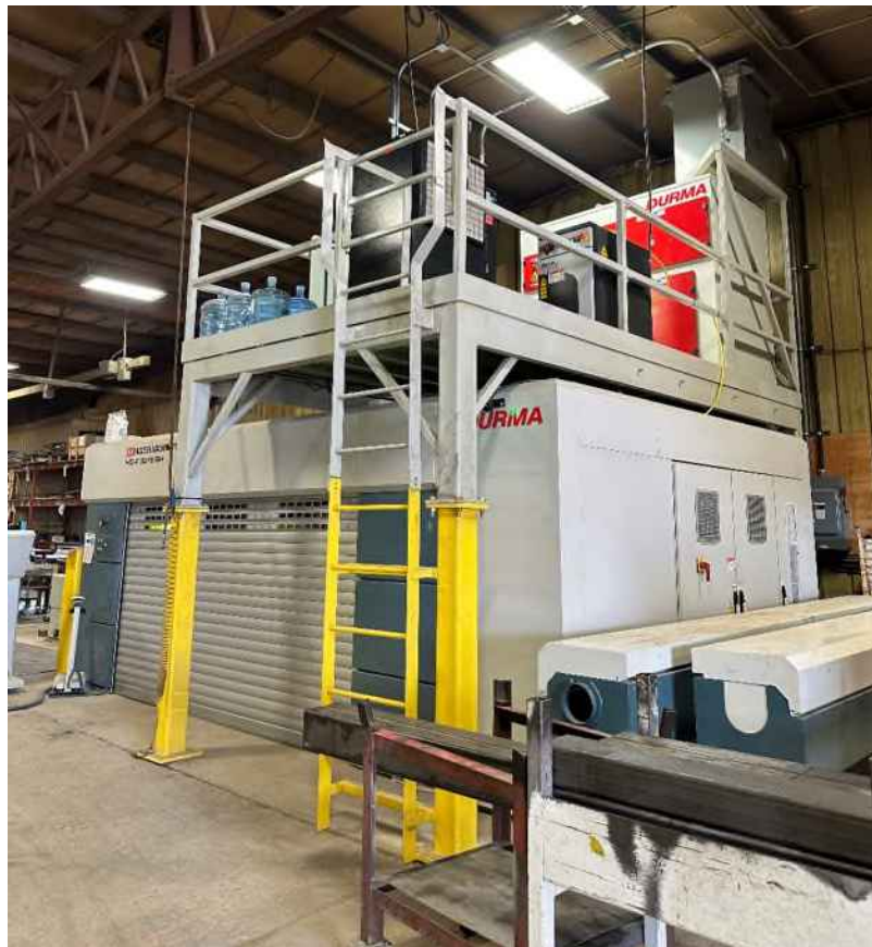
Photo 16: General view of Bystronic laser cutting machine. (Tetra Tech, June 2023)
