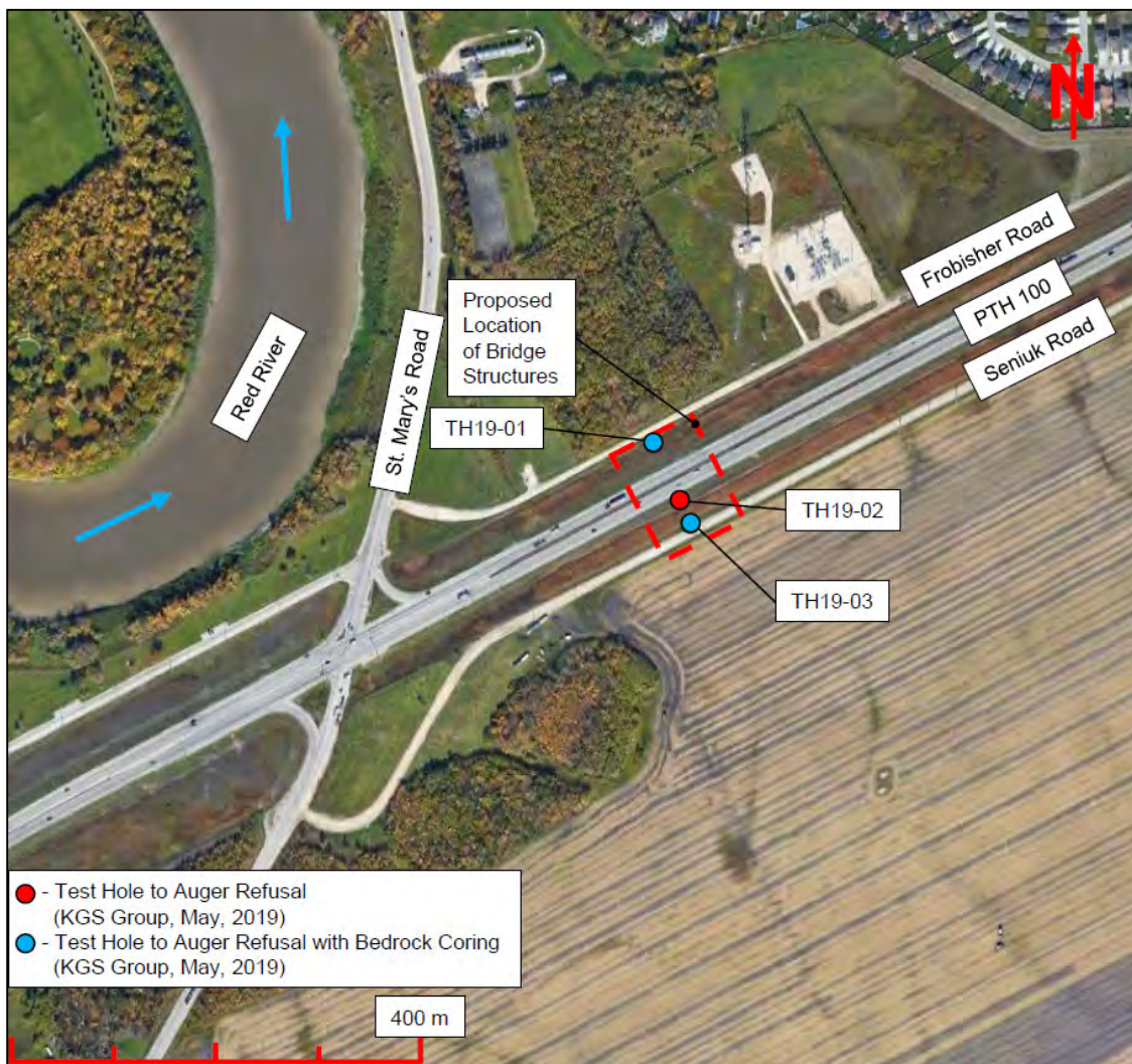
Figure 4. Geotechnical Investigation - Site Plan
