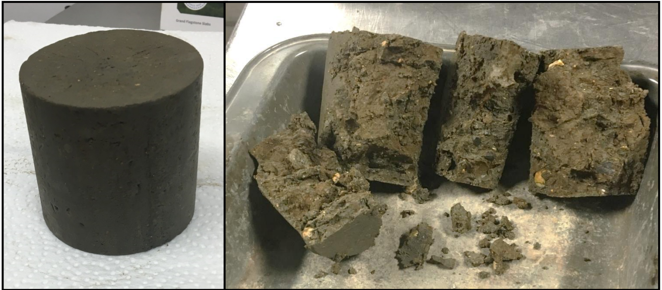
PHOTOGRAPH #5: Sample TH1-S5 after hydraulic conductivity testing.
