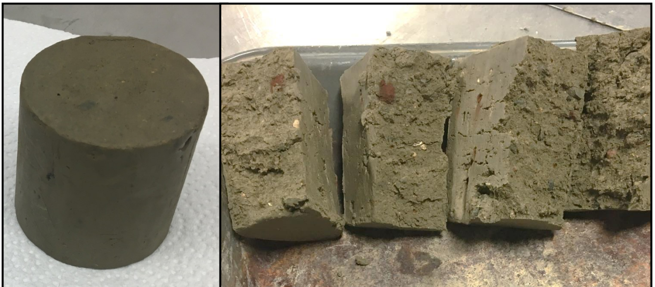
PHOTOGRAPH #6: Sample TH4-S2 after hydraulic conductivity testing.
