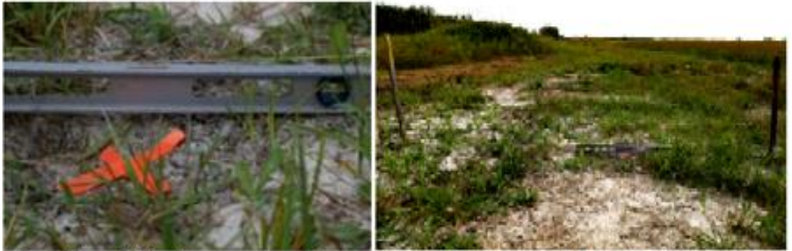
Figure 20 a and b Surface expression of abandoned sealed CanWhite borehole near Ross Manitoba in a slight depression (no mounding) with clay sealing on top of the cut off borehole.
