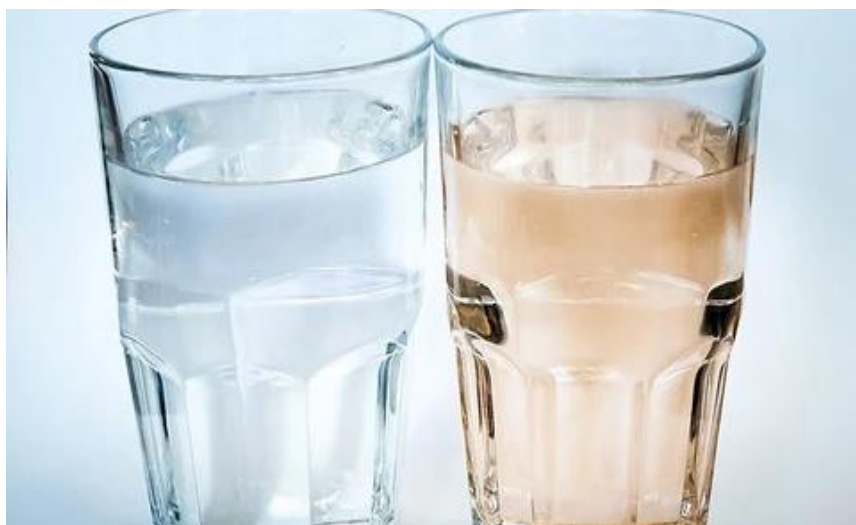
Figure 11. Unoxidized (left) and oxidized (right) manganese in well water. Source:
