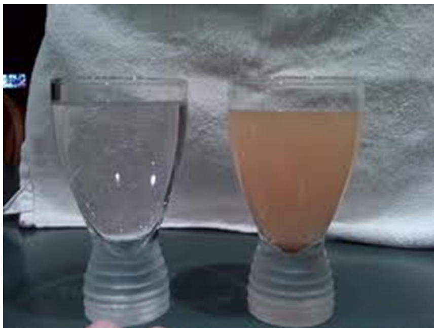
Figure 10. Iron-containing well water without (left) and with (right) oxygen.
