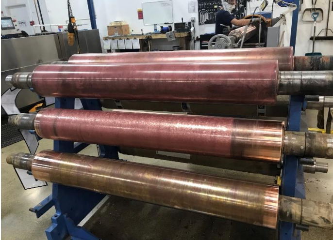
Photo 3: Steel cylinders plated with copper
