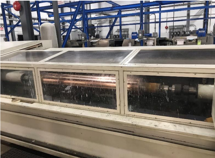
Photo 4: Steel cylinder that is being polished for Electro Engraving
