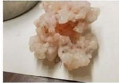
Figure 2. Selective Solution Mining In this illustration the potash has been extracted by dissolution and the salt remains.
