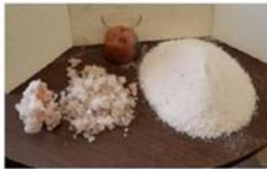
Figure 3. Potash 62% K 2 O/99.5% KCl The white pile is the dissolved potash that has been crystalized. This quantity of potash came from the actual potash ore.
