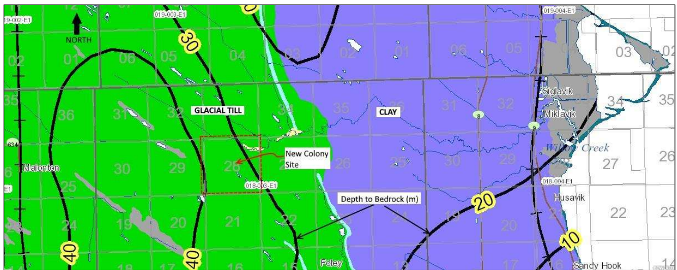
Figure 3 – Surficial geology (plan view); contours indicate depth to bedrock (m). (Source – Manitoba Mineral Resources, 2013)
