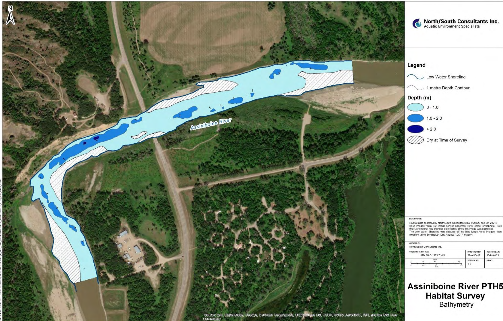
Figure 2. Bathymetric map of the PTH 5 Bridge survey area on the Assiniboine River near Glenboro, Manitoba.
