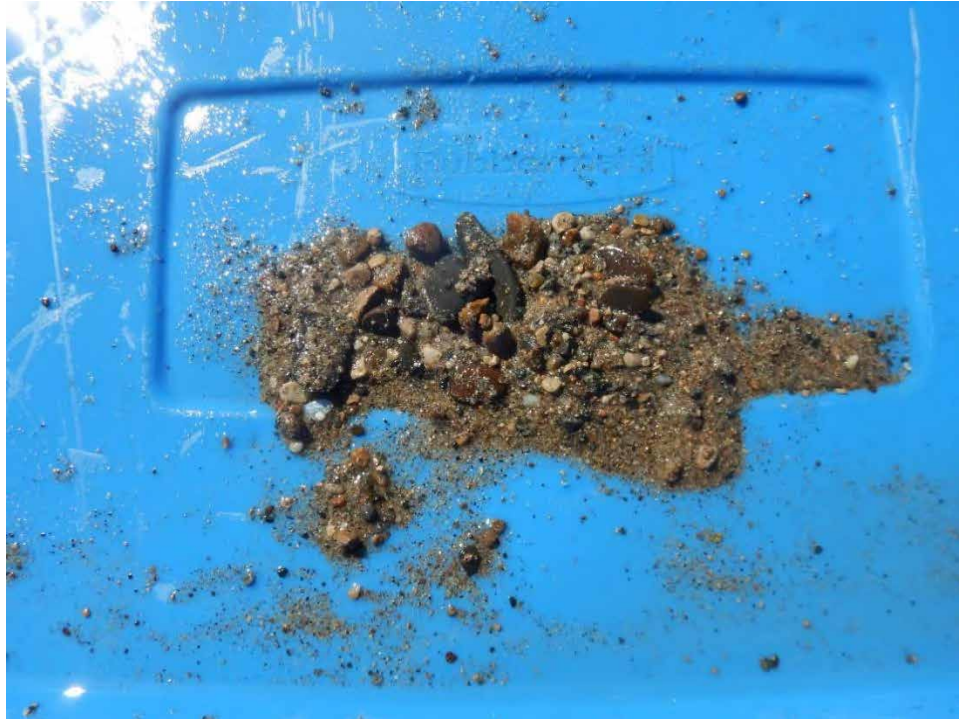
Photo 13. Substrate validation from Site 7 at the PTH 5 bridge survey area, showing a gravel/sand substrate.
