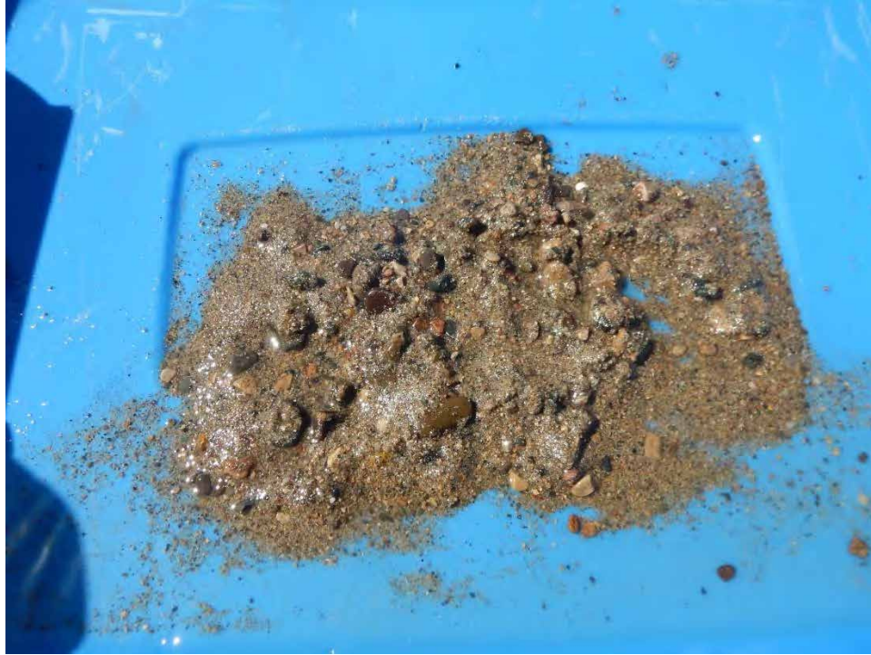
Photo 15. Substrate validation from Site 9 at the PTH 5 bridge survey area, showing a sand/gravel substrate.
