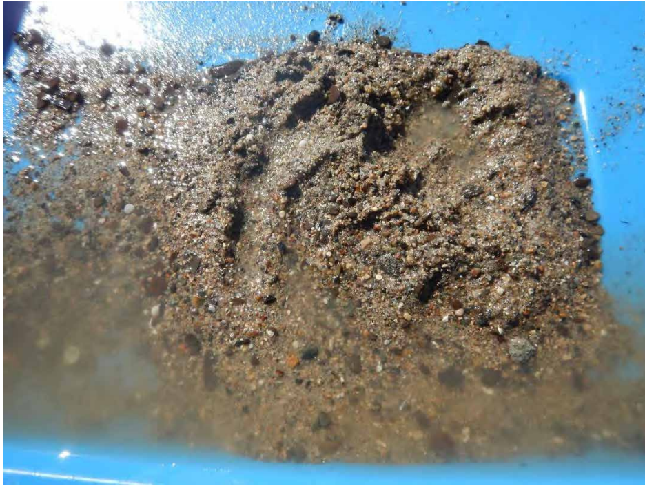
Photo 31. Substrate validation from Site 29 at the PTH 5 bridge survey area, showing a sand/gravel/silt substrate.
