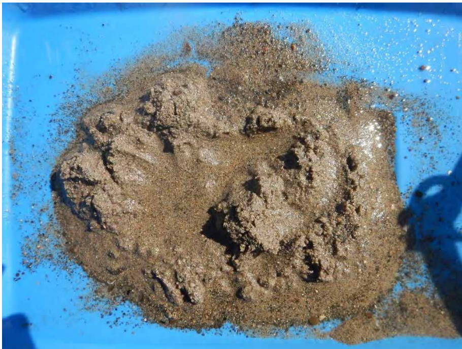
Photo 42. Substrate validation from Site 40 at the PTH 5 bridge survey area, showing a sand/gravel substrate.
