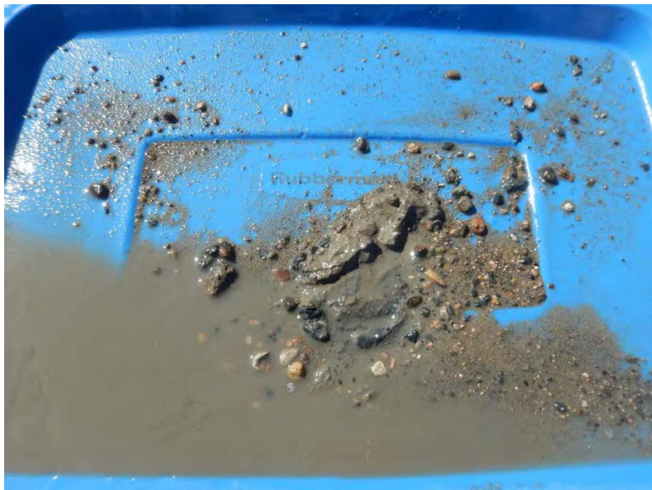
Photo 32. Substrate validation from Site 30 at the PTH 5 bridge survey area, showing a sand/gravel/clay substrate.
