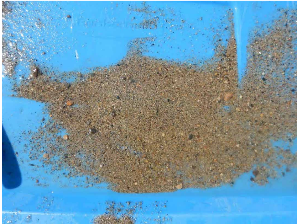
Photo 11. Substrate validation from Site 5 at the PTH 5 bridge survey area, showing a sand/gravel substrate.
