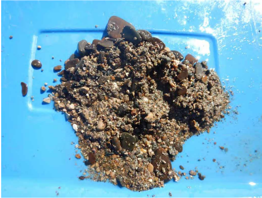
Photo 41. Substrate validation from Site 39 at the PTH 5 bridge survey area, showing a gravel/sand substrate.
