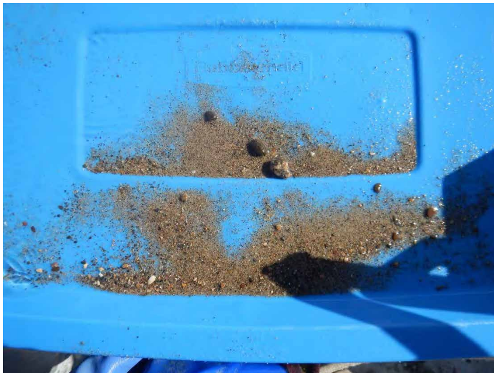
Photo 46. Substrate validation from Site 44 at the PTH 5 bridge survey area, showing a sand/gravel substrate.
