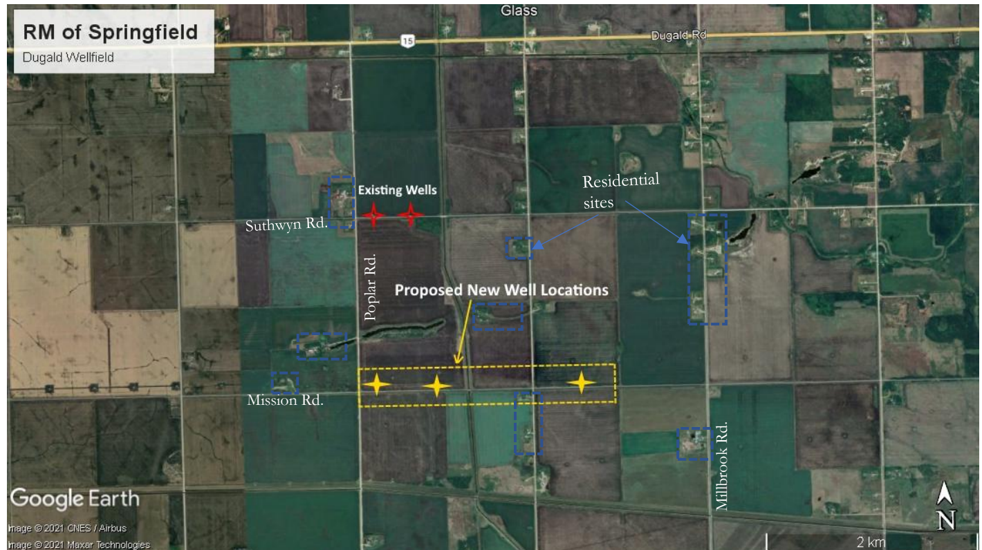
Figure 4 – Proposed locations (approximate) for additional pumping wells (yellow); existing wells plotted in red; existing residential noted in blue. (Source – Google Earth, 2021)
