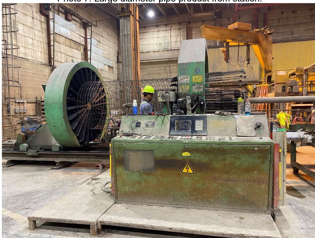
Photo 8. Rebar cage welding station.
