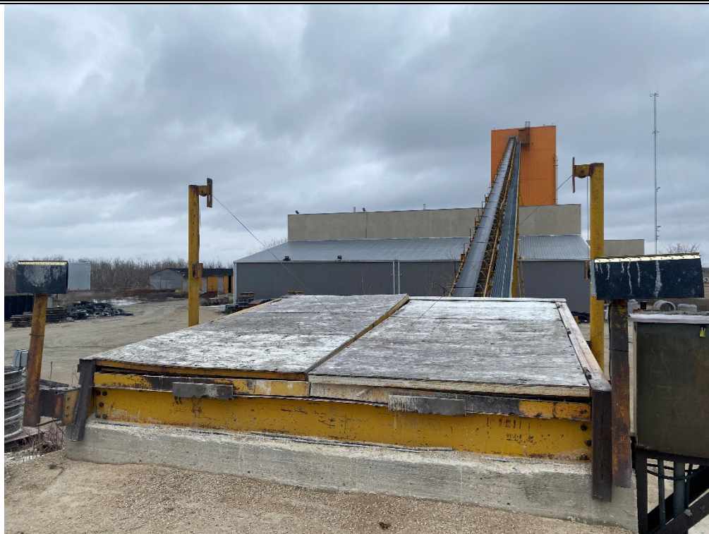
Photo 1. Aggregate loading hopper and belt conveyor in background.
