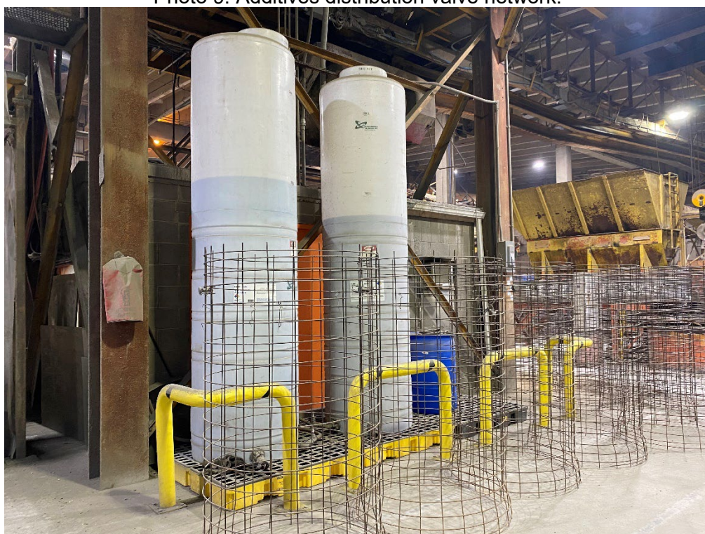
Photo 10. Additive bulk storage (2 x 2500 L and 1 x 205L).
