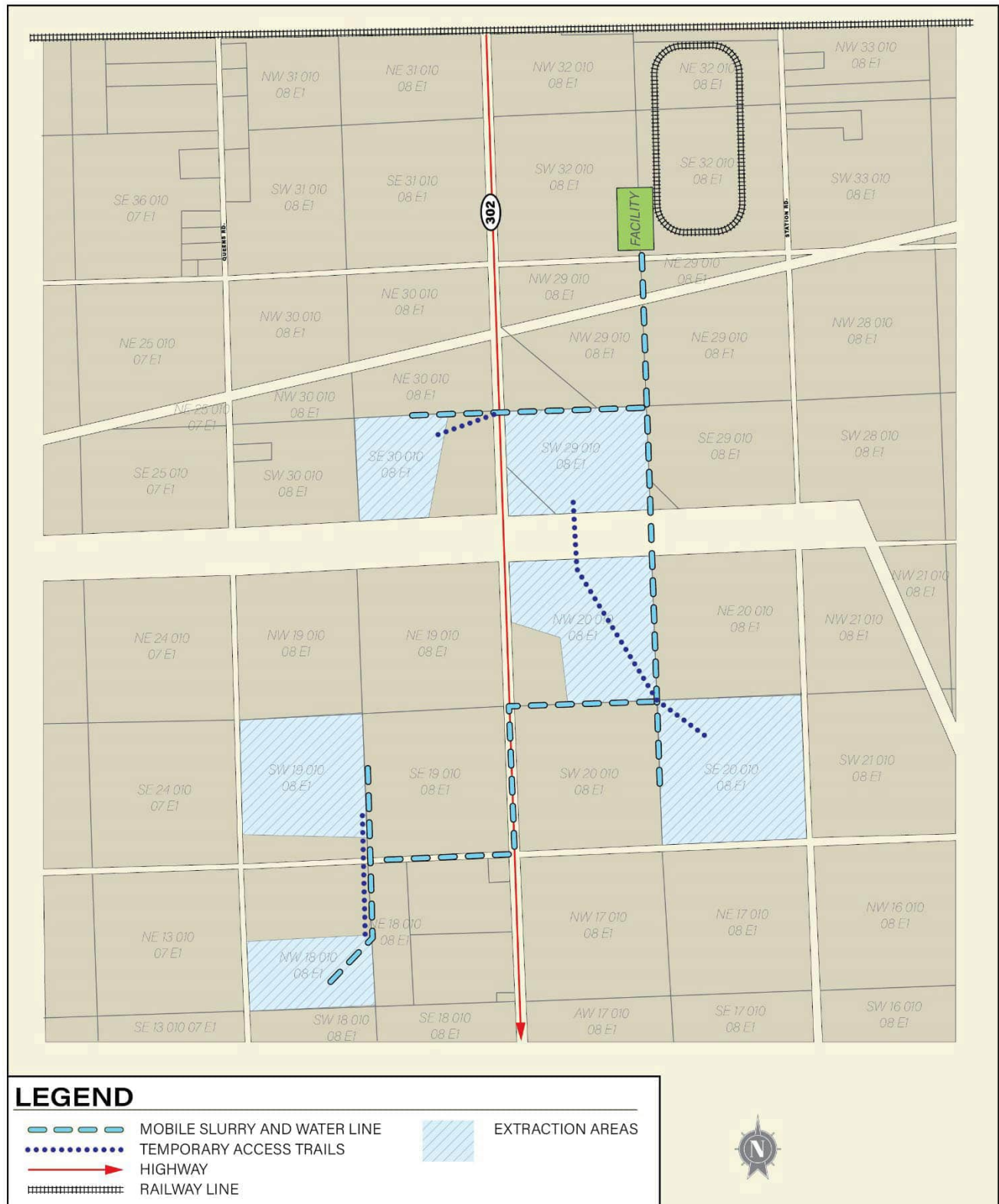
Figure 2-5: General layout of Mobile Slurry and Water Lines and Temporary Access Trails
