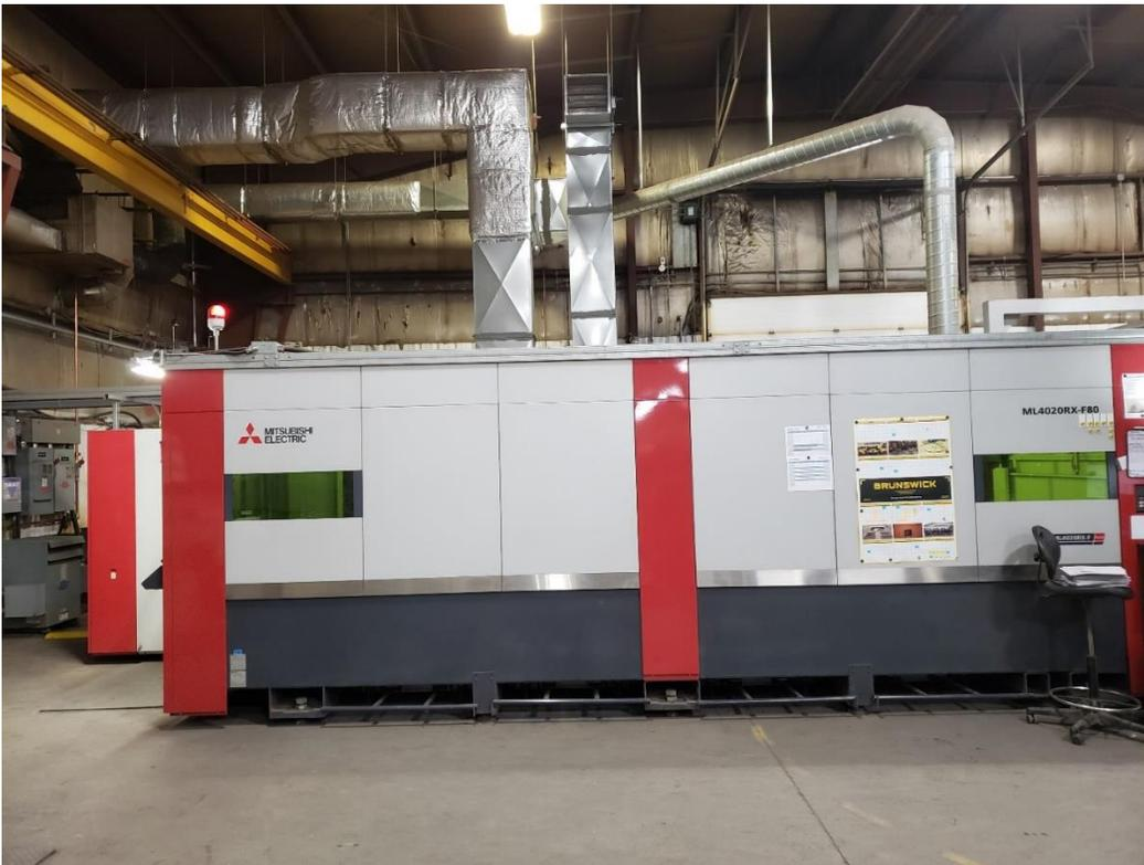
Figure 2 - Example 2 of Additional Equipment for Expansion – Flat Sheet Laser
