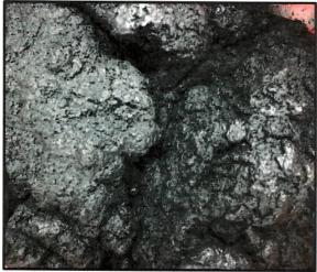
Photograph 1: City of Winnipeg dewatered biosolids used in the 2019 bench-scale soil fabrication trial (March, 2019).
