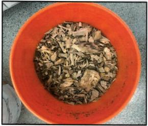
**Photograph 2:** Woodchips used in the 2019 bench-scale soil fabrication trial (March, 2019).
