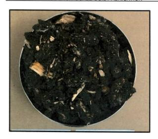
Photograph 7: Mix 3, blended at room temperature using the mechanical soil mixer (March, 2019).
