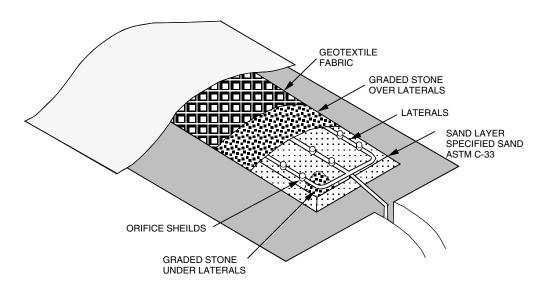
NOTE: INTENDED FOR >60%-100% HEAVY CLAY SOILS \*FOR ILLUSTRATIVE PURPOSE ONLY, NOT TO SCALE NOTE: ALL SEPTIC FIELDS MUST BE BERMED WITH SUITABLE MATERIAL.
