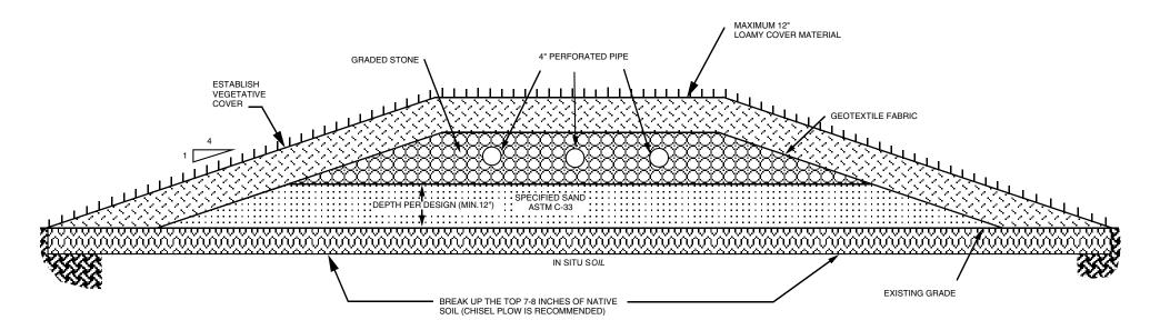
NOTE: INTENDED FOR > 60%-100% HEAVY CLAY SOILS \*FOR ILLUSTRATIVE PURPOSE ONLY, NOT TO SCALE NOTE: ALL SEPTIC FIELDS MUST BE BERMED WITH SUITABLE MATERIAL.
