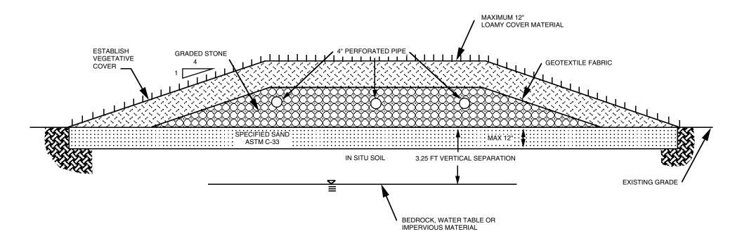
NOTE: INTENDED FOR 40-60% CLAY SOILS \*FOR ILLUSTRATIVE PURPOSE ONLY, NOT TO SCALE NOTE: ALL SEPTIC FIELDS MUST BE BERMED WITH SUITABLE MATERIAL.
