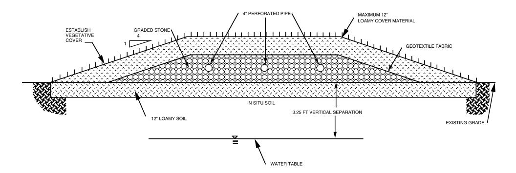
NOTE: INTENDED FOR 85-100% SAND \*FOR ILLUSTRATIVE PURPOSE ONLY, NOT TO SCALE NOTE: ALL SEPTIC FIELDS MUST BE BERMED WITH SUITABLE MATERIAL.
