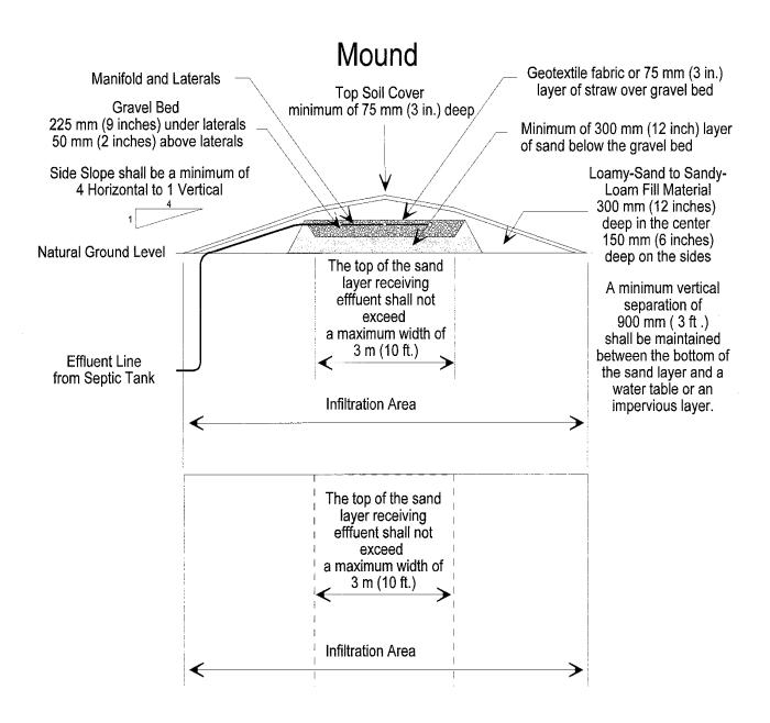
Pressurized Sand Treatment Mound Note: Wastewater Effluent Chambers may also be used. Intended for use in heavy clay soils \*for illustrative purposes only, not to scale
