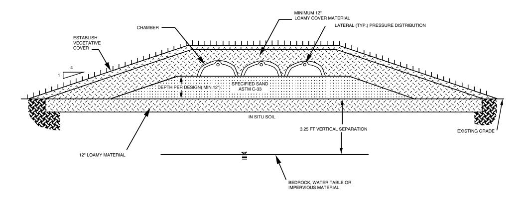
NOTE: INTENDED FOR 85%-100% SAND \*FOR ILLUSTRATIVE PURPOSE ONLY, NOT TO SCALE NOTE: ALL SEPTIC FIELDS MUST BE BERMED WITH SUITABLE MATERIAL.
