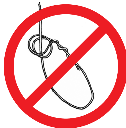
Figure 2 - Prohibited Traditional Double-loop Knot
