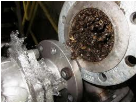
A three-foot-diameter pipe clogged by zebra mussels in less than three months (U.S. Department of Energy)
