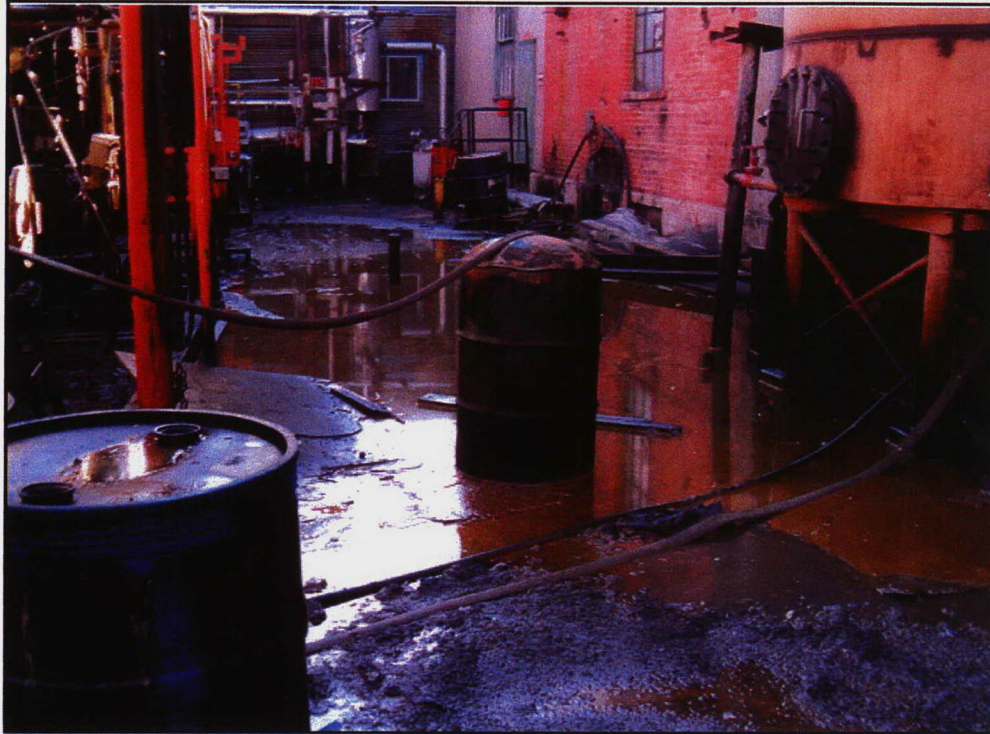
PHOTOGRAPH #35: View of an apparent oil spill along the east side of Building E.
