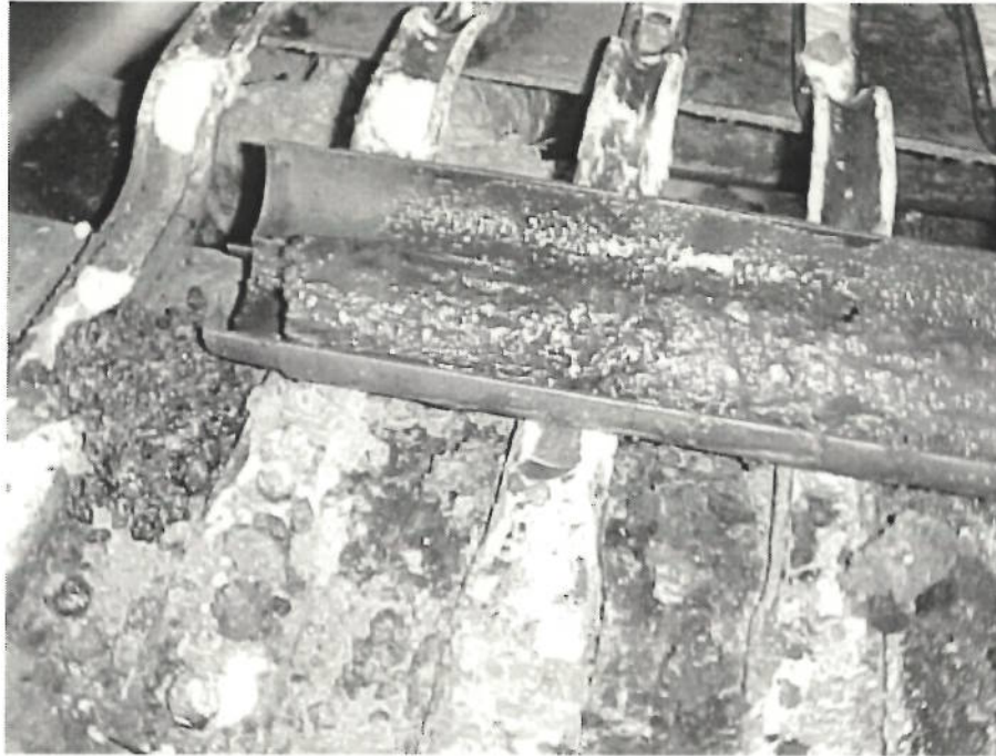
A sheen was often evident on the outside of contaminated soil samples when the split spoons were opened
