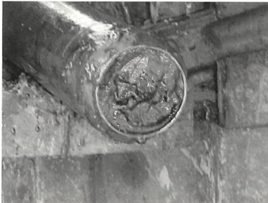
Liquid coal tar residue observed at end of split spoon sampler.
