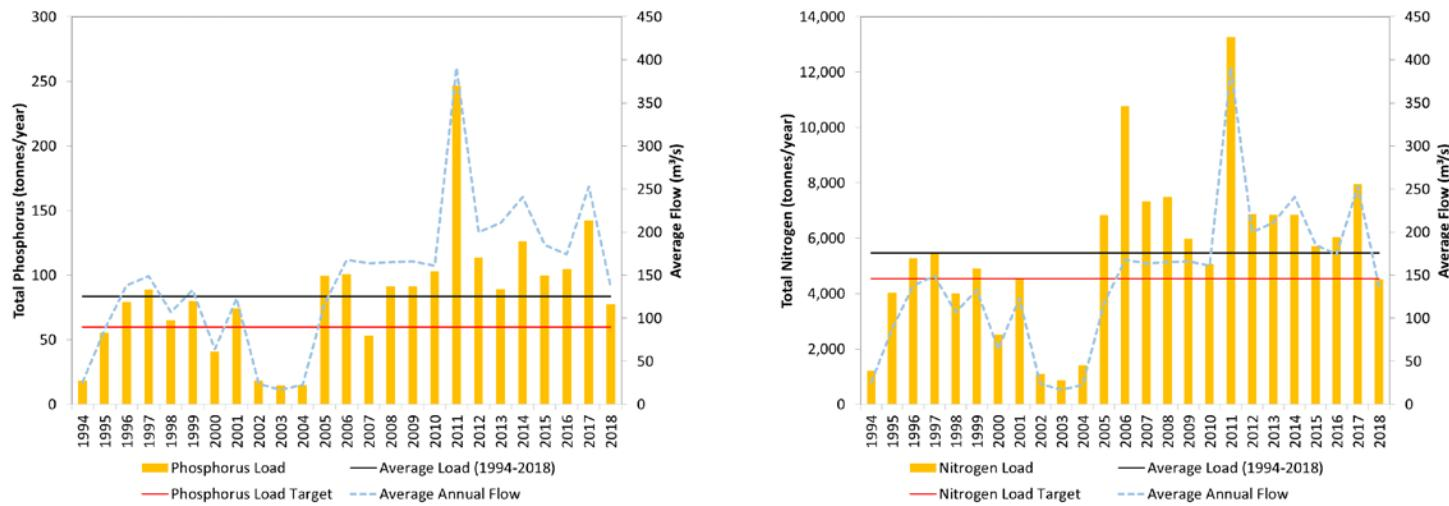
Figure 5. Annual total phosphorus and total nitrogen loads (tonnes/year) and flows in the Dauphin River (upstream of Anama Bay), 1994 to 2018 compared to the proposed nutrient loading targets.
