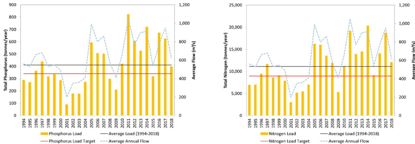
Figure 4. Annual total phosphorus and total nitrogen loads (tonnes/year) and flows in the Saskatchewan River (at Grand Rapids), 1994 to 2018 compared to the proposed nutrient loading targets.
