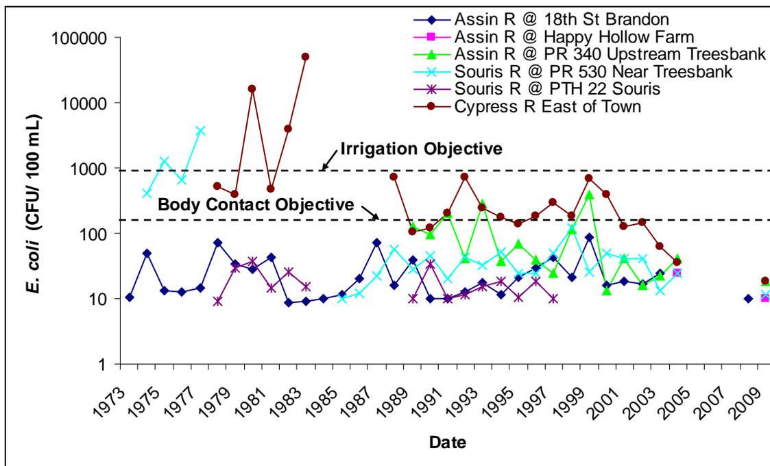
Figure 14: Densities of *Escherichia coli* (*E. coli*) collected from six long term water quality monitoring sites in the Central Assiniboine watershed between 1970 and 2009. The objective is 200 MPN per 100 mL.
