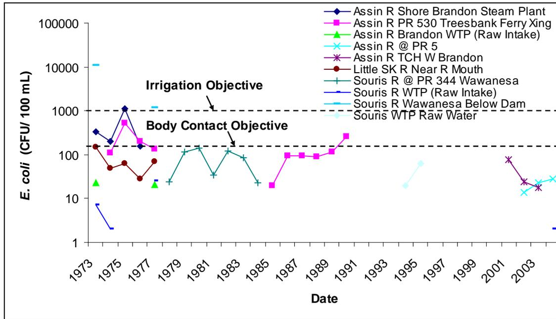
Figure 15: Densities of *Escherichia coli* (*E. coli*) collected for 10 other monitoring sites, not part of the long term water quality monitoring program, in the Central Assiniboine watershed between 1970 and 2009. The objective is 200 MPN per 100 mL.
