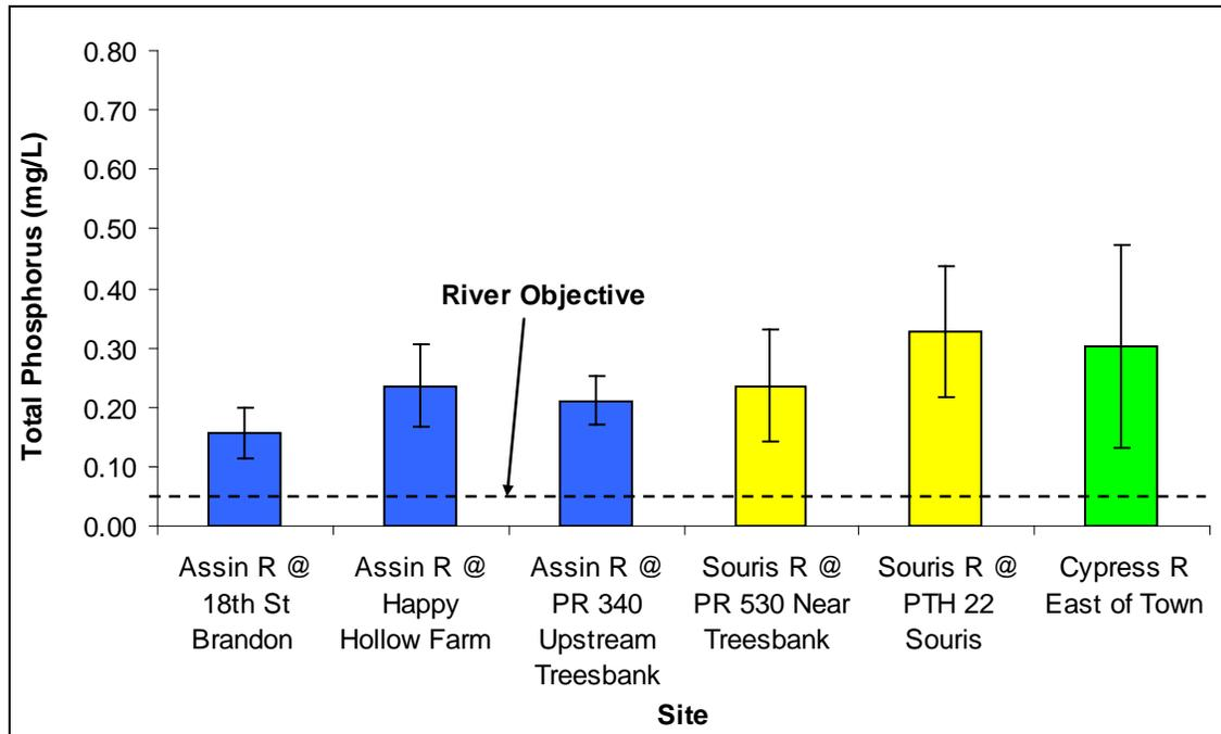
Figure 7: Mean total phosphorus concentrations (mg/L) between 1970 and 2009 for six long term water quality monitoring sites.
