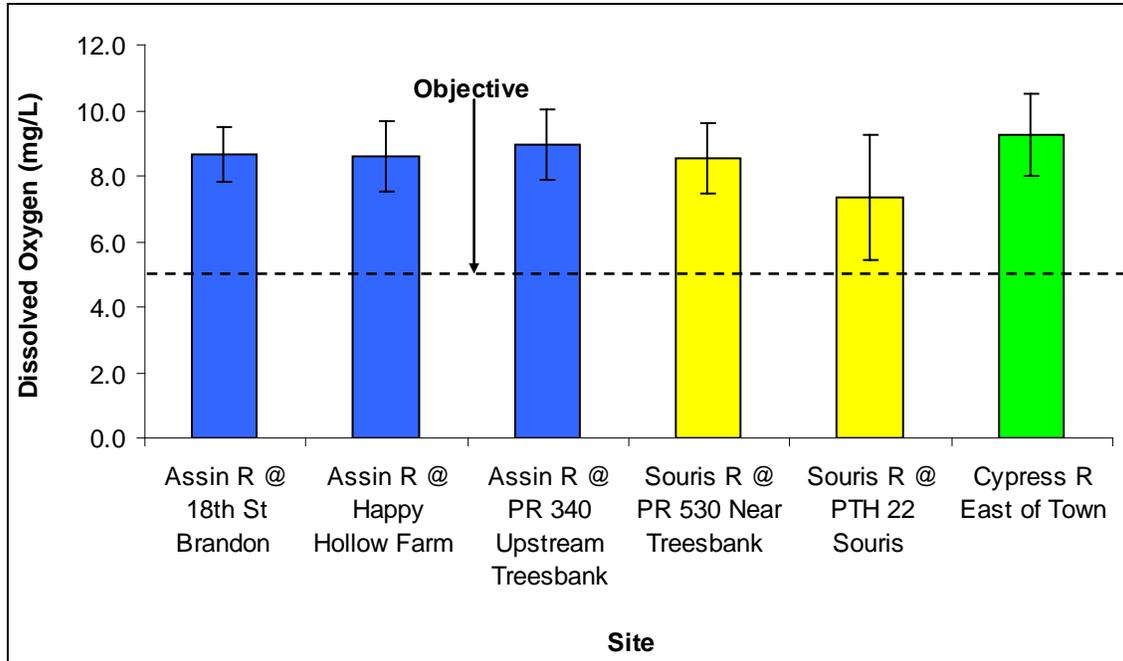
Figure 13: Mean dissolved oxygen (mg/L) concentrations between 1970 and 2009 for six long term water quality monitoring sites.
