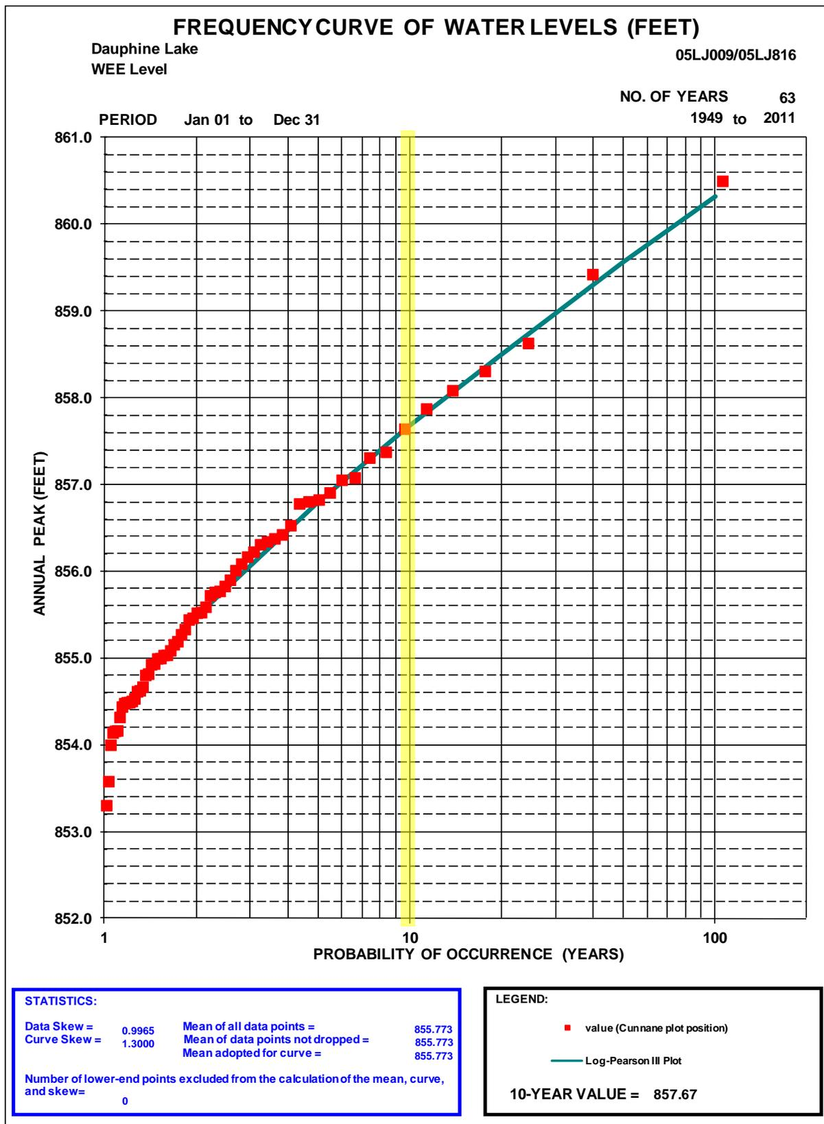
Figure 9: Frequency curve of peak wind-eliminated water levels of Dauphin Lake
