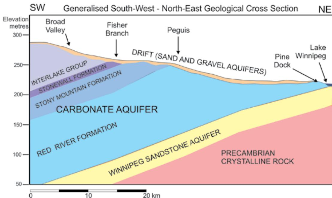
Figure 2: Generalized Regional Cross Section of Aquifers located within the Fisher River Watershed
