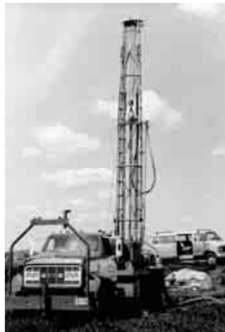
Well drilling equipment, used for both test drilling and well construction.
