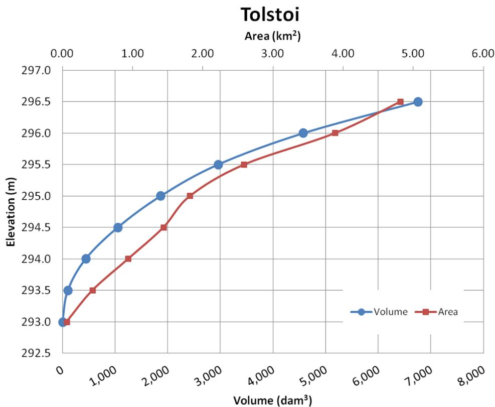
**Figure 39:** Tolstoi Retention Elevation-Volume-Area curves
