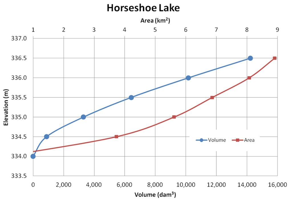
**Figure 11:** Horseshoe Lake Retention Elevation-Volume-Area curves
