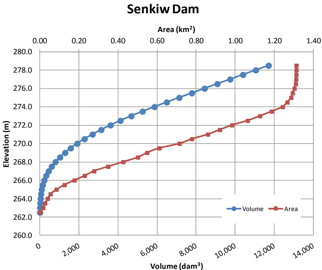
**Figure 32:** Senkiw Dam Retention Elevation-Volume-Area curves
