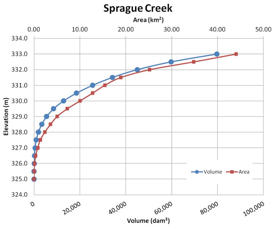
Figure 42: Sprague Creek Retention Elevation-Volume-Area curves
