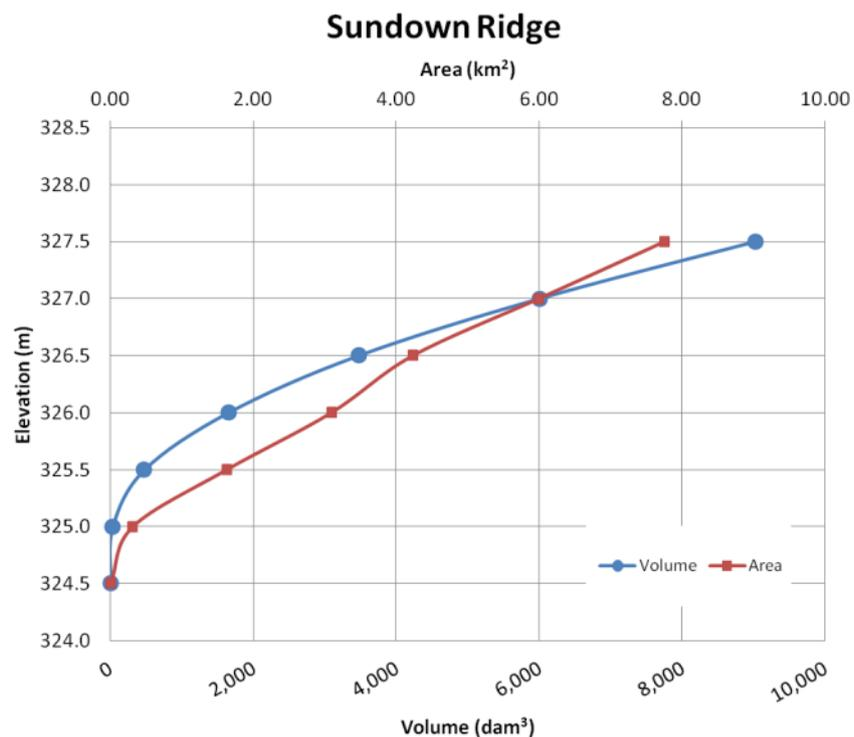
Figure 15: Sundown Ridge Retention Elevation-Volume-Area curves
