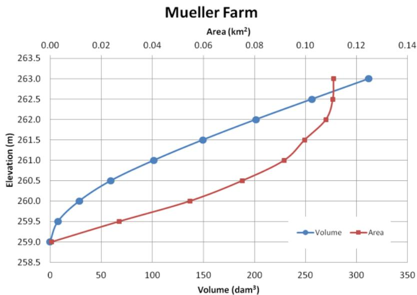
Figure 19: Mueller Farm Retention Elevation-Volume-Area curves
