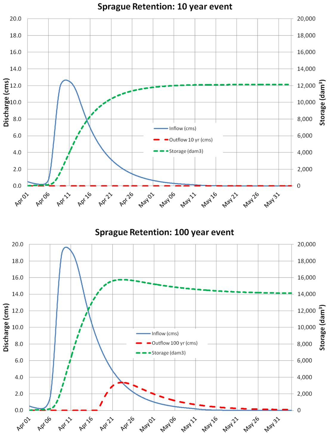
**Figure 44: Sprague Retention Effects**
