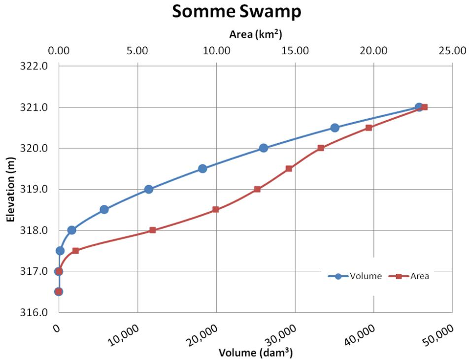
**Figure 36:** Somme Swamp Retention Elevation-Volume-Area curves
