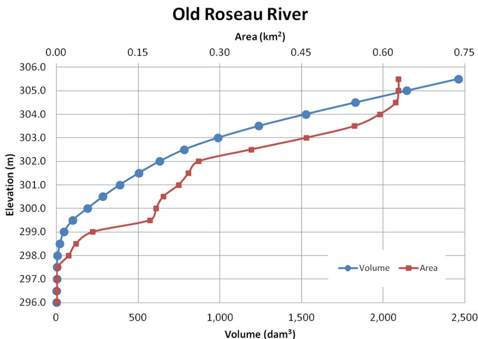
**Figure 29:** Old Roseau River Retention Elevation-Volume-Area curves
