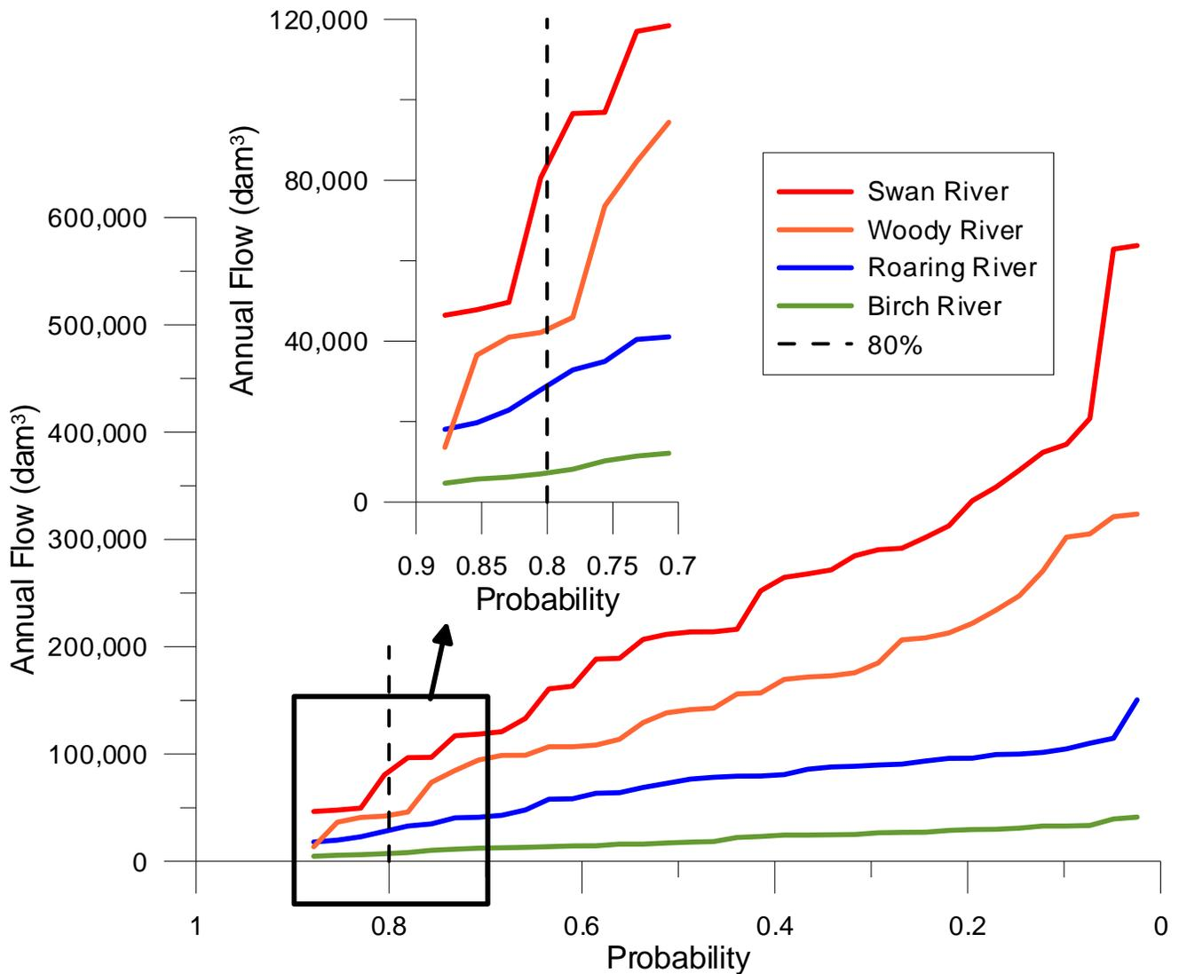
Figure 15: Flow duration curves at the gauges on Swan, Roaring, Woody and Birch rivers for the time series 1973 – 2009. Water production is taken to be the flows that are not exceeded 80% of the time.
