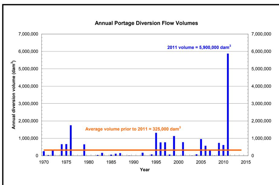
The Portage Diversion was completed in 1970. It is one component of the works constructed in the 1960's to prevent flooding in Winnipeg. The Diversion consists of two separate control structures: one which controls the flows down the Assiniboine River and another which diverts some of the flow of water in the Assiniboine River into a 29 km long diversion channel that empties into Lake Manitoba near Delta Beach. The diversion was originally designed to carry a maximum flow of 700 m<sup>3</sup>/s.
