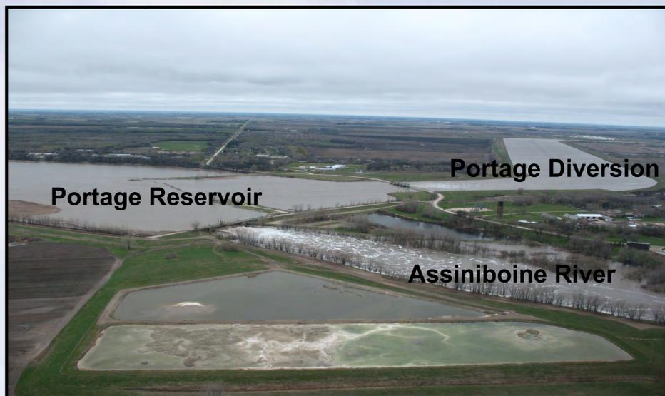
Portage Diversion on May 11, 2012 when the flow into the Portage Reservoir was 1,412 m<sup>3</sup>/s and 862 m<sup>3</sup>/s was being diverted into Lake Manitoba.
